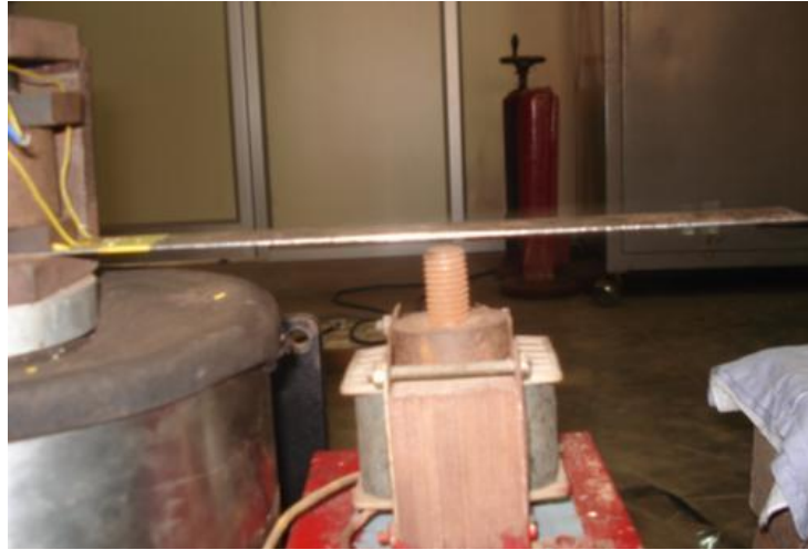
Plate 4.2 Magnetic shaker below the cantilever
