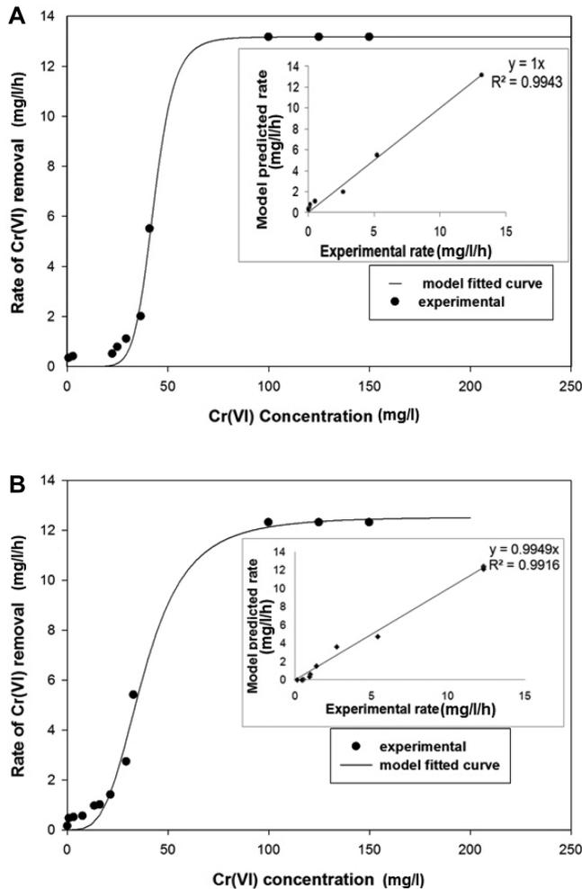
**Fig. 3.** Rate of Cr(VI) removal (mg/l/h) vs. Cr(VI) concentration (mg/l) (A) with Cr-B2 grown in nutrient media; and (B) with Cr-B2 grown in LB media.
