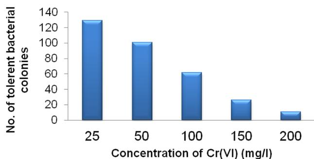
**Fig. 1.** Tolerant bacterial colonies number obtained during screening of Cr(VI)-resistant bacteria under each level of Cr(VI) concentration.
