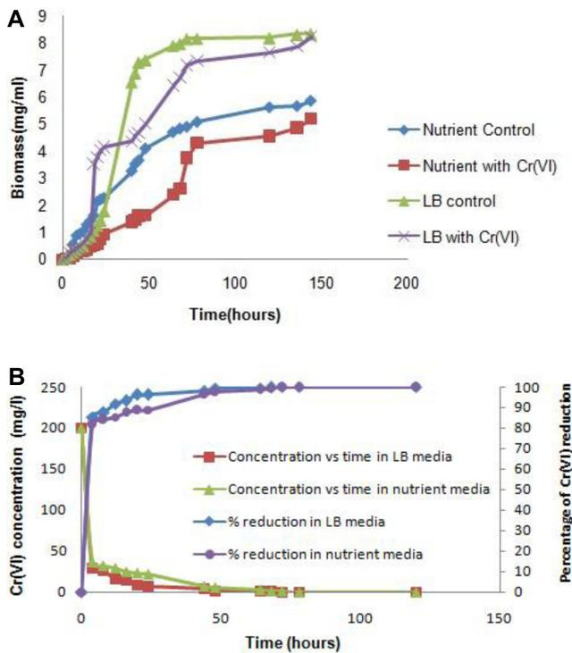
**Fig. 2.** Effect of media on Cr-B2 growth and Cr(VI) reduction. (A) Growth profile of Cr-B2 under nutrient media and LB media in the absence and presence of Cr(VI). (B) Time course variation of Cr(VI) concentration and the percentage Cr(VI) reduction in the presence of LB and nutrient media with Cr-B2.
