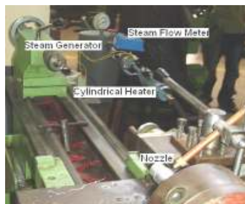
Figure 5. Steam generator and steam feeding system.
