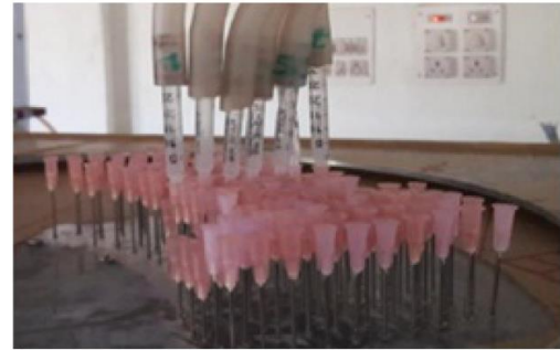
Fig. 7. Static pressure tapping arrangement on the top end wall.
