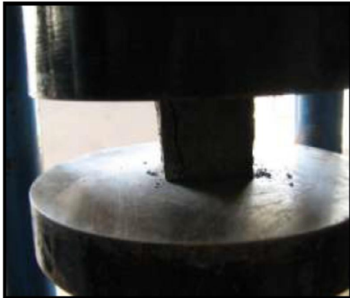
Figure 5: Compression Testing of Cement Mortar Cubes
