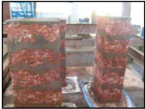
Figure 7: Laterite Masonry Prisms Cast for Testing
