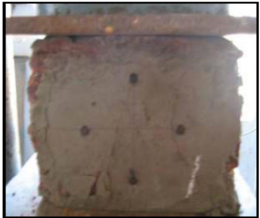
Figure 3: Demec Buttons Glued in Laterite Blocks to Measure Strains
