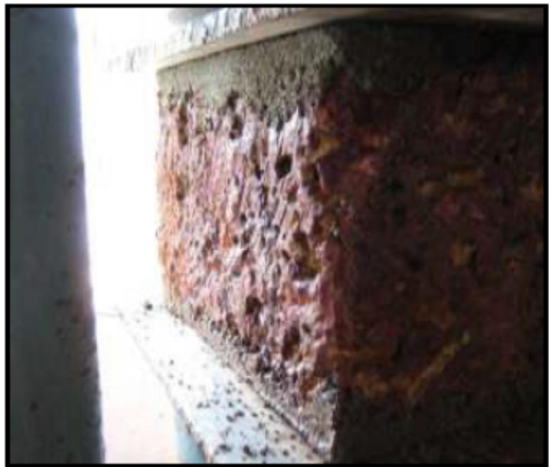
Figure 1: Laterite Block Capped with Cement Mortar for Compression Test
