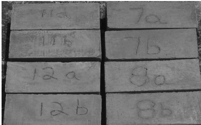
Figure 5 Bricks with IOT, sand and cement (see online version for colours)
