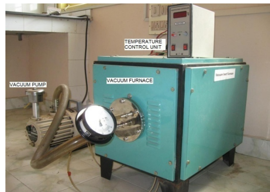
Figure-6. Vacuum furnace used for sintering.
