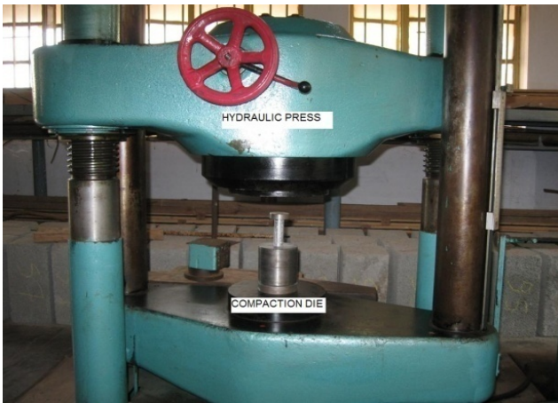
Figure-3. Compaction setup.
