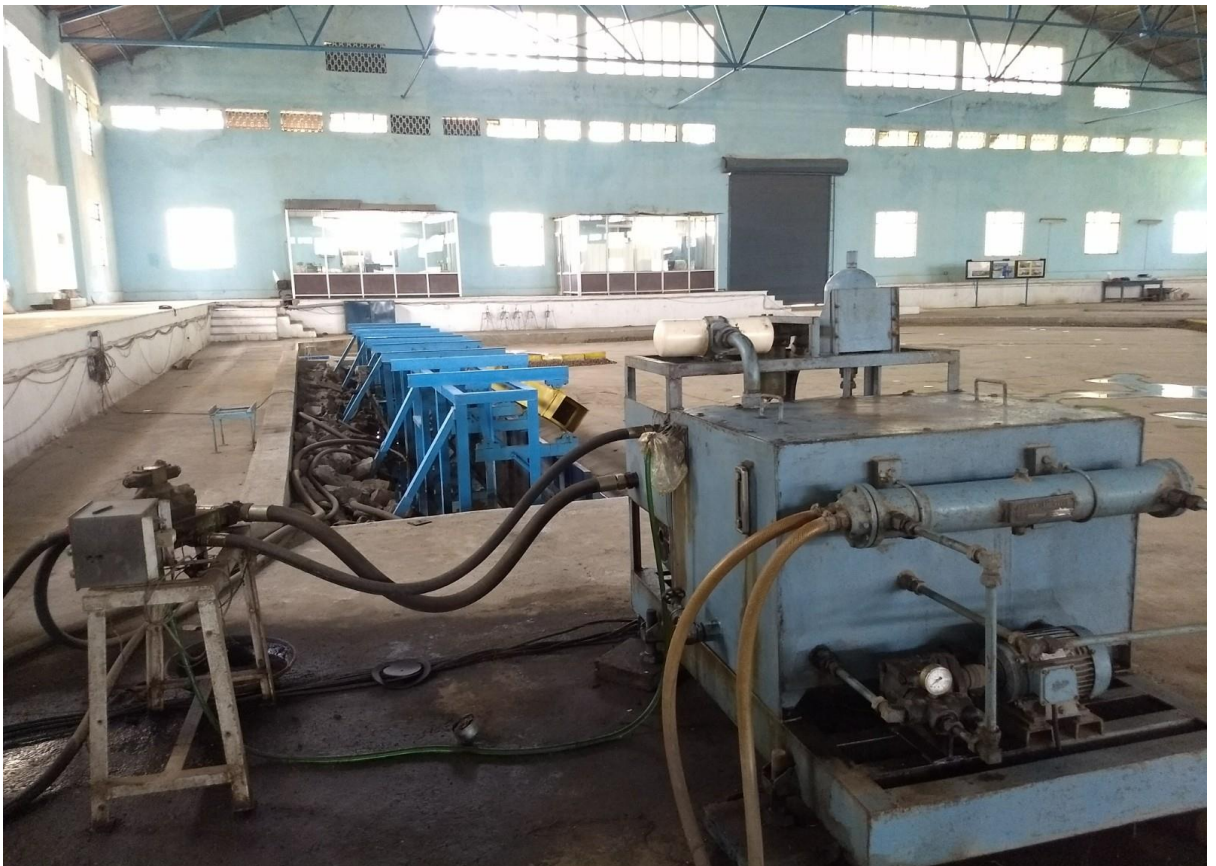
Plate 3.4 Hydraulic power pack with servo control system.
