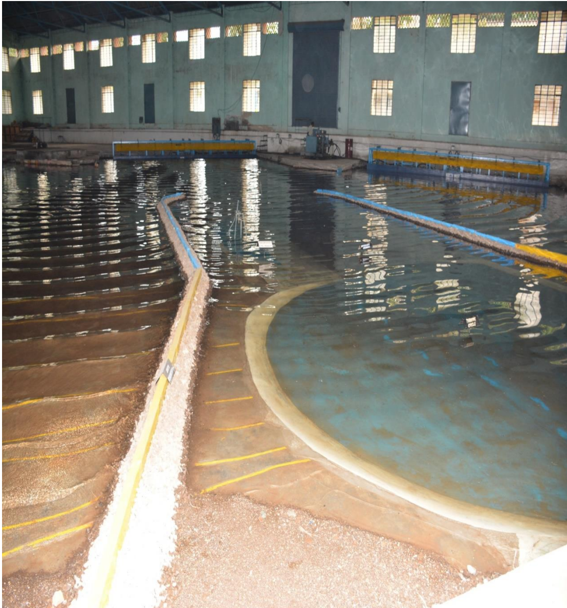
Plate 4.7 Wave propagation with extension of breakwater with curved tips
