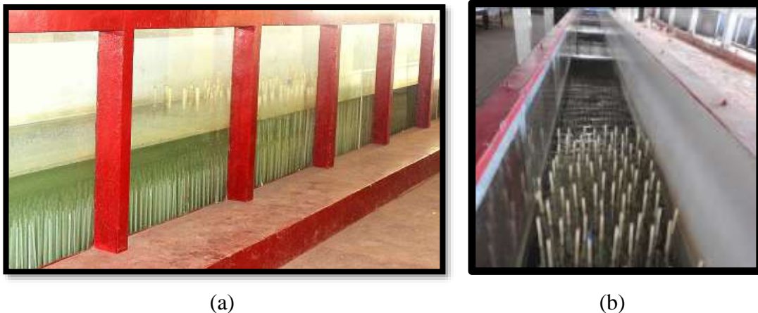
Plate 6.2 Snapshots of wave propagation along the emergent heterogeneous model a) side view b) top view
