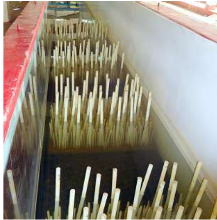
Fig. 3.15 Photo of model setup to study wave attenuation over fragmented emergent trunk model with roots
