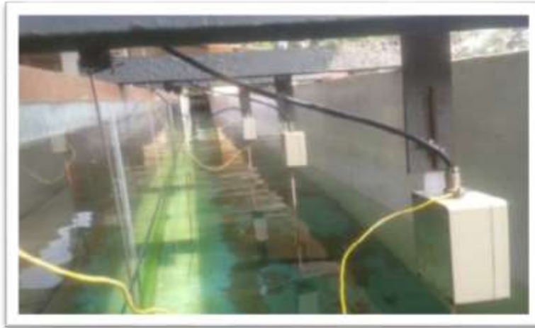
Plate 3.2 Arrangement of wave probes for data acquisition
