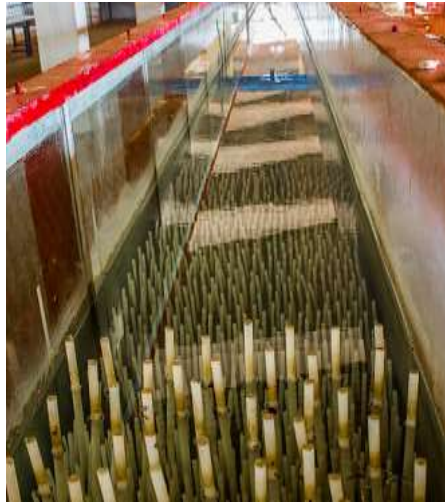
Fig. 3.14 Photo of model setup to study wave attenuation over a compound heterogeneous model (top view)
