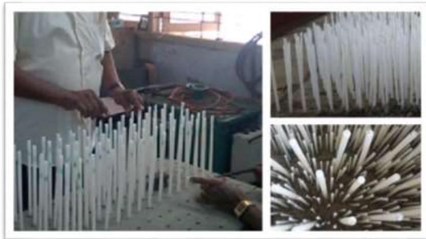
Plate 3.6 Fixing the simulated vegetation model on to the base slab
