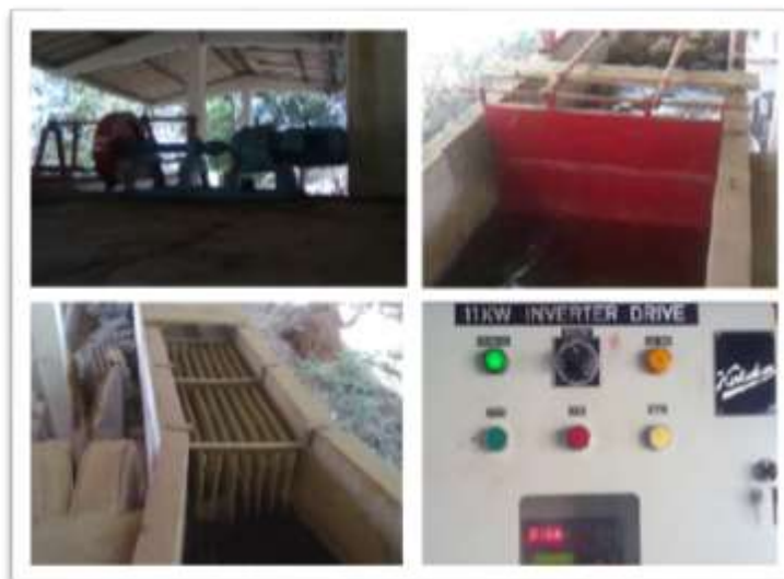
Plate 3.4 Wave generating system (clockwise from top left: motor, flap type wave paddle, inverter drive, wave filter)
