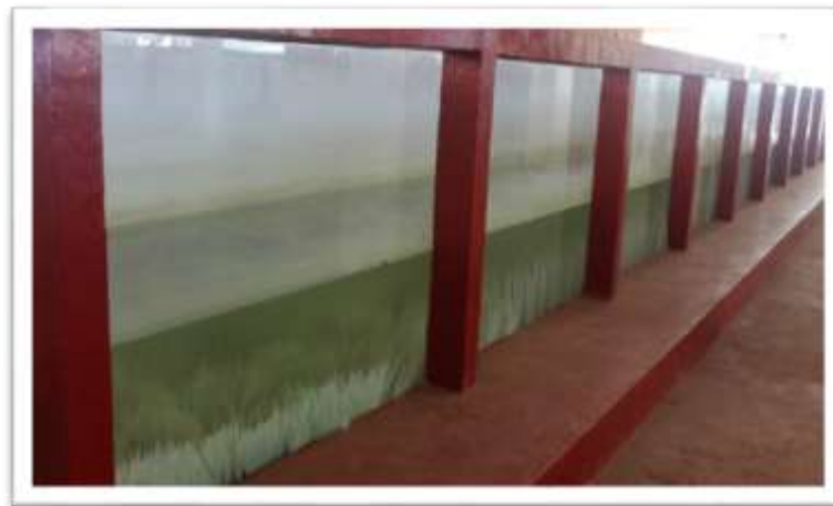
Plate 3.1 View of wave flume with the simulated vegetation placed on the flume bed
