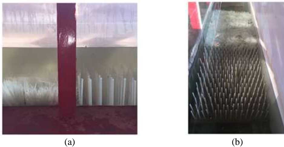
Fig. 3.12 Photo of model setup to study wave attenuation over a submerged heterogeneous vegetation model a) Side view b) Top view
