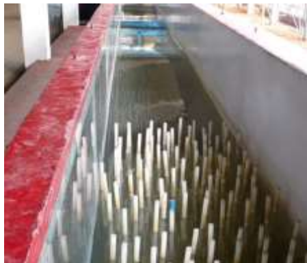
Fig. 3.16 Photo of model setup to study wave attenuation over a fragmented compound heterogeneous model
