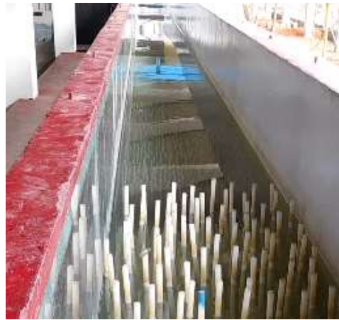
Fig. 3.13 Photo of model setup to study wave attenuation over a emergent heterogeneous model (top view)
