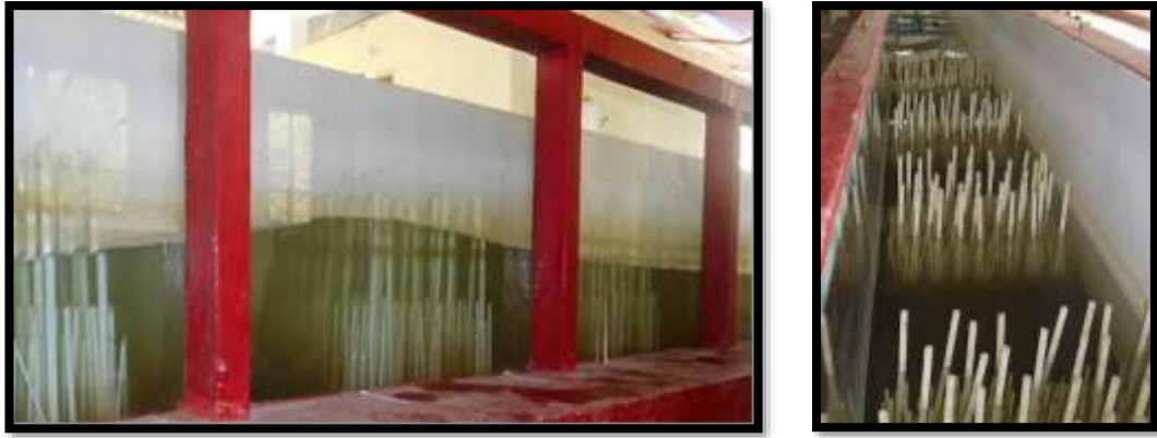
Plate 7.1 Snapshots of model setup to study wave attenuation over a fragmented emergent trunk model with roots a) Side view b) Top view
