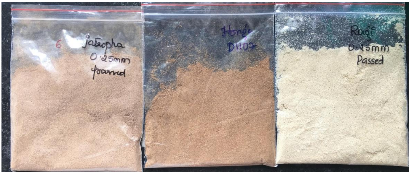
untreated fibers of d) Jatropha seed shell e) Pongamia seed shell f) Finger millet straw.
