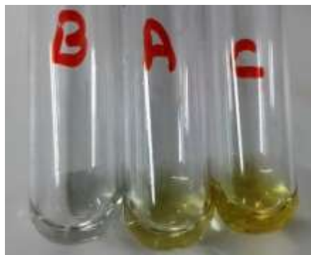
Figure 4.18: Ellman's reaction performed for native uricase and Uc-mPEG-mal conjugates. (Test-tube B contains blank buffer, Test-tube A contains Ellman's reaction mixture for Uc-mPEG-mal conjugates and Test-tube C contains Ellman's reaction mixture for native uricase)
