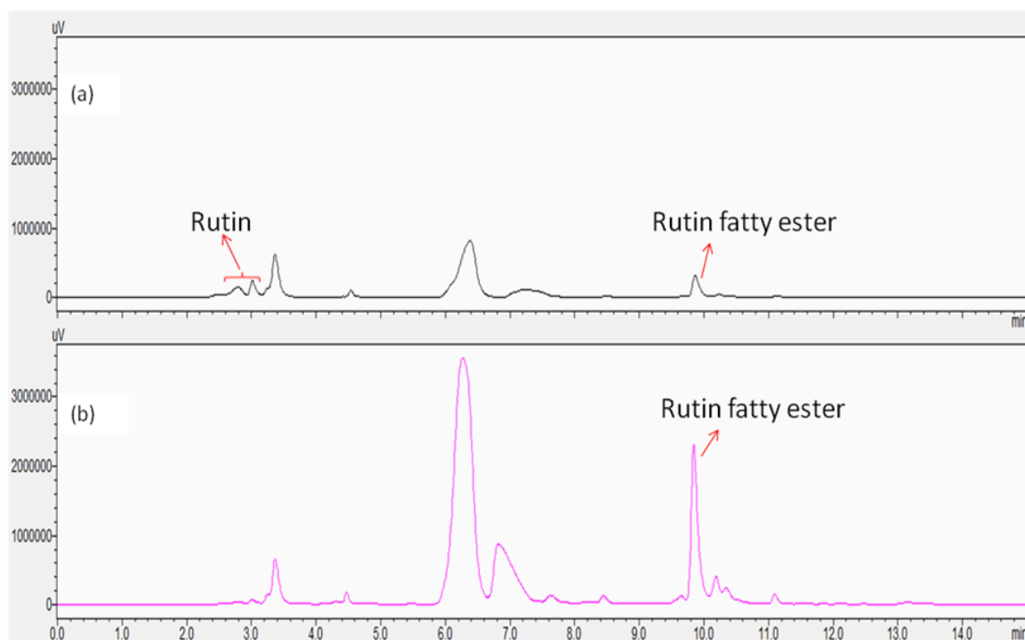
Figure 5.11 HPLC chromatogram of rutin and rutin fatty ester (a) before purification and (b) after purification by using ethyl acetate: water
