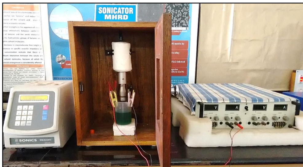
Figure 3.5 – Experimental setup used for deposition of monolayer and multilayer alloy coating, under different conditions of sonication at constant c.d. using DC Power source (Aplab, LD3205) and Ultrasound generator (SONIC Vibra-Cell™ VC 750)
