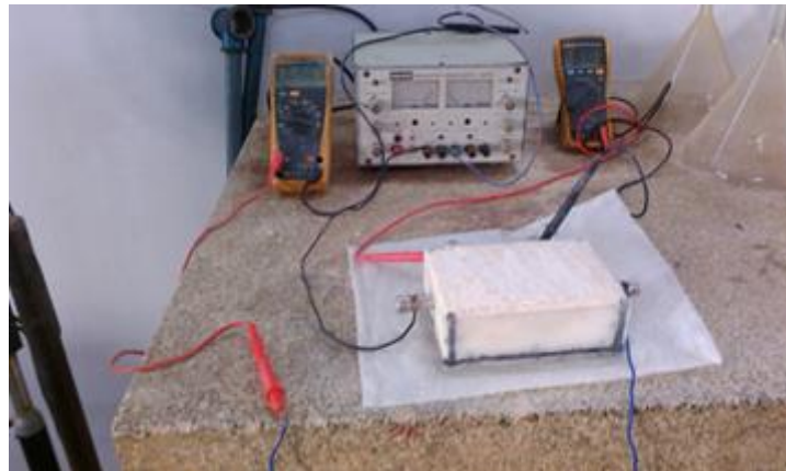
Figure 3.7 Soil resistivity measurement
