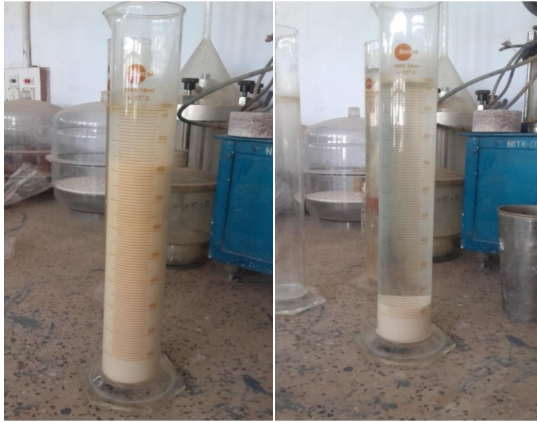
Figure 7.11 Hydrometer test for contaminated soil (a) just after mixing (b) one hour later
