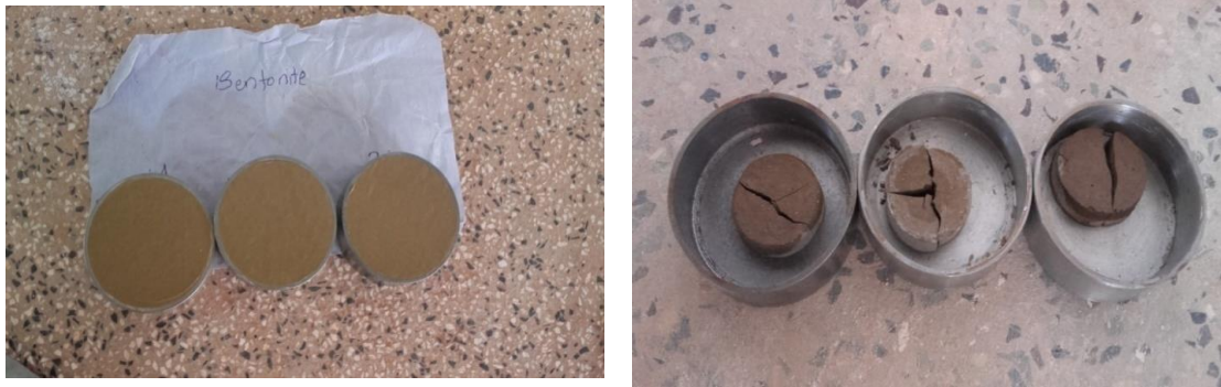
Figure 7.49 Pure bentonite shrinkage pats (a) wet state and (b) After air and oven drying
