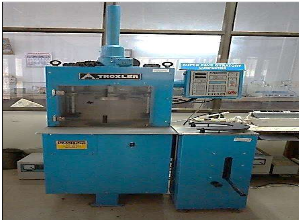
Fig.3.2. Superpave gyratory compactor
