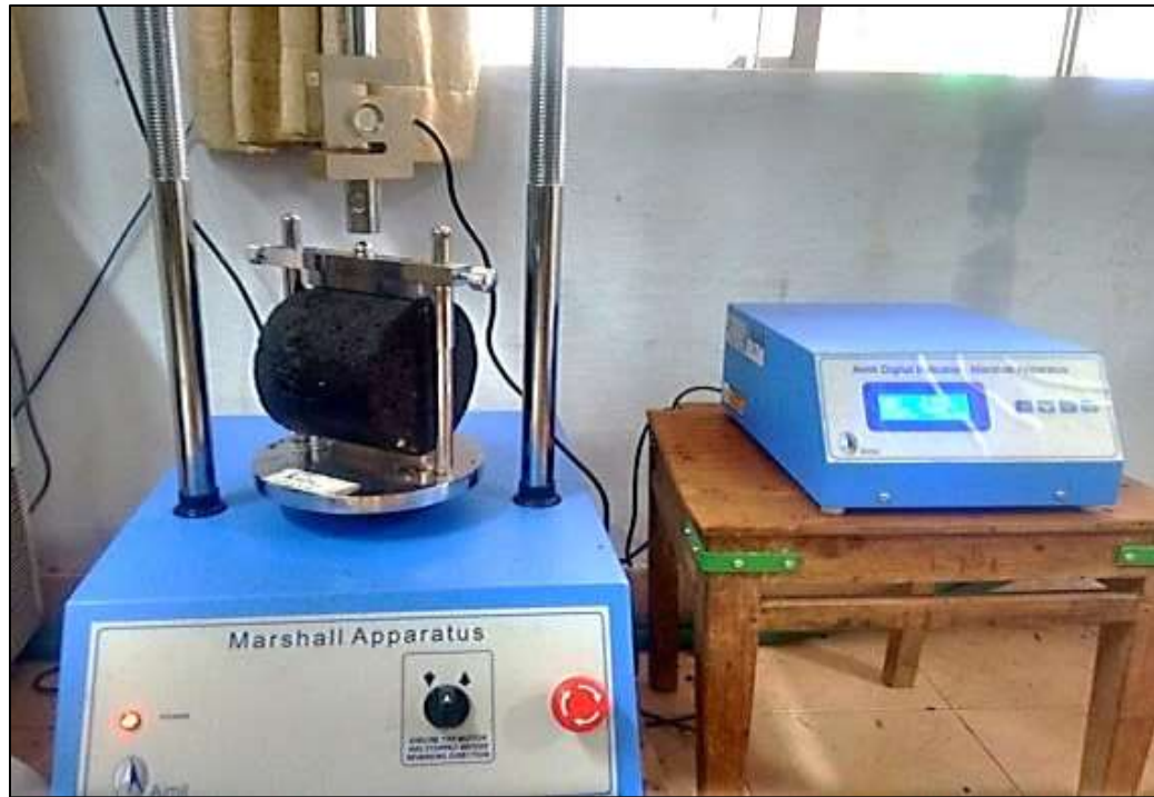
Fig. 3.5. Indirect tensile strength test setup
