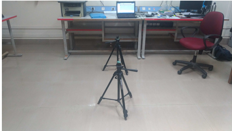
Figure 3.17: RSSI fluctuation at height 0.5334m to 1.33m using tripod
