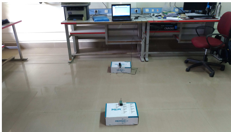
Figure 3.14: RSSI fluctuation at height 0.10m
