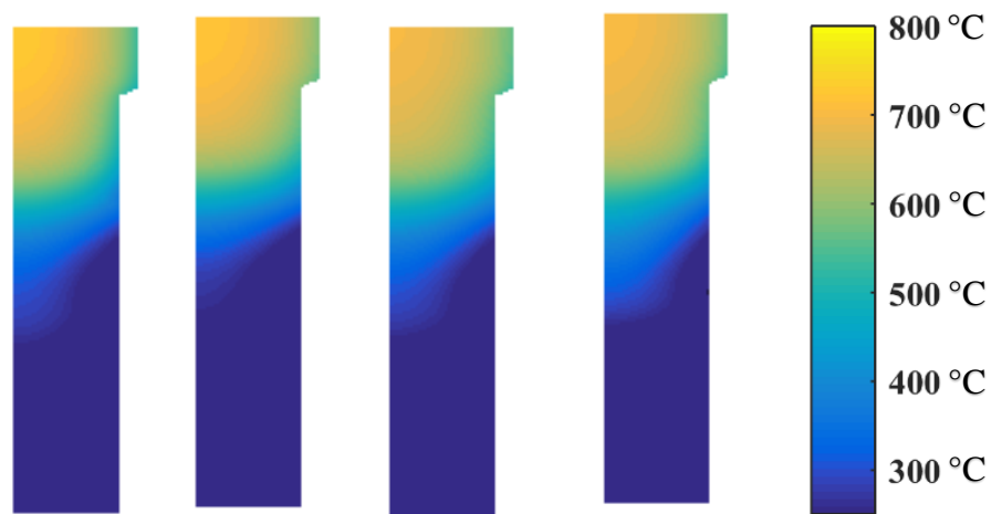
Figure 5.10: Thermal profile in Inconel alloy during quenching in CuO nanofluids of concentrations 0.01, 0.05, 0.1 and 1.0 vol.% (from left to right) at average surface temperature of 250 °C
