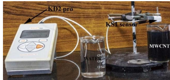
Figure 3.8: Photograph of KD2 pro with KS1 sensor for measuring thermal conductivity of liquid media
