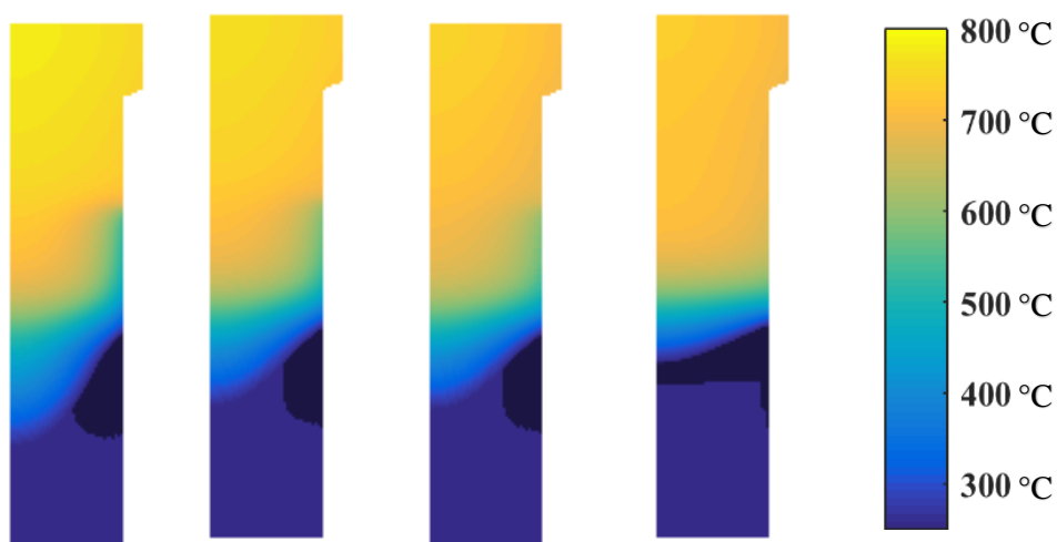
Figure 5.9: Thermal profile in Inconel alloy during quenching in CuO nanofluids of concentrations 0.01, 0.05, 0.1 and 1.0 vol.% (from left to right) at average surface temperature of 440 °C
