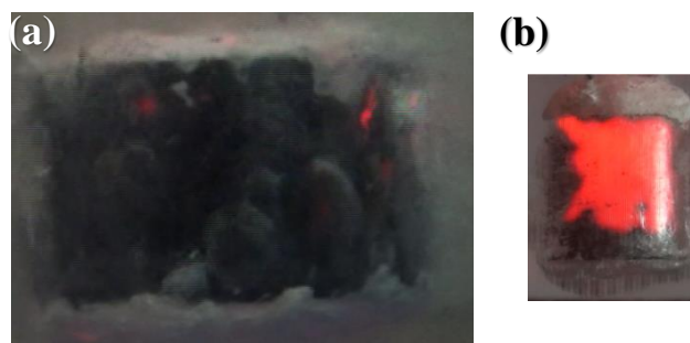
Figure B.3: Video image taken during quenching of steel probes of (a) 50 and (b) 25 mm in distilled water
