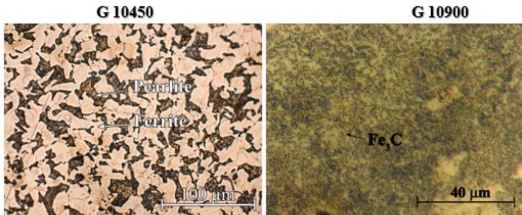
Figure 4.10: As-rolled microstructure of G 10450 and G 10900 steel alloys
