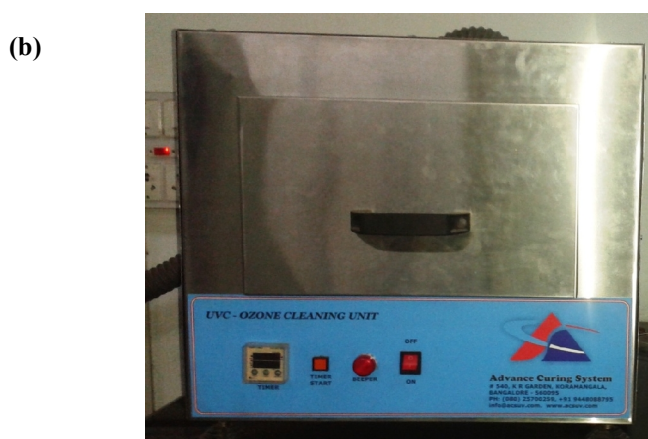
Figure 2.1 (b) UV-O 3 chamber
