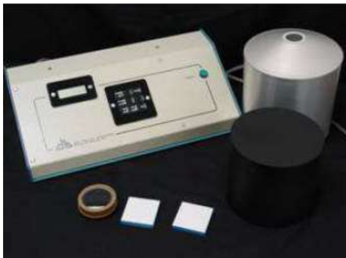
Figure 2.3: Photograph of the solar spectrum reflectometer (SSR).
