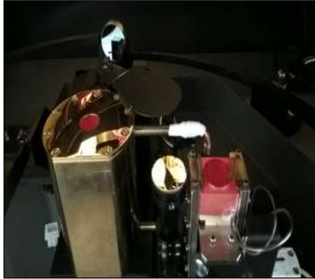
Figure 6.3: Photograph of the measurement set up. From left to right, blackbody IR source at 700°C with chopper, reference sample (specular gold), heated sample holder with Sample 1 at set-point of 500°C. The movable detecting mirror is also visible in the back.
