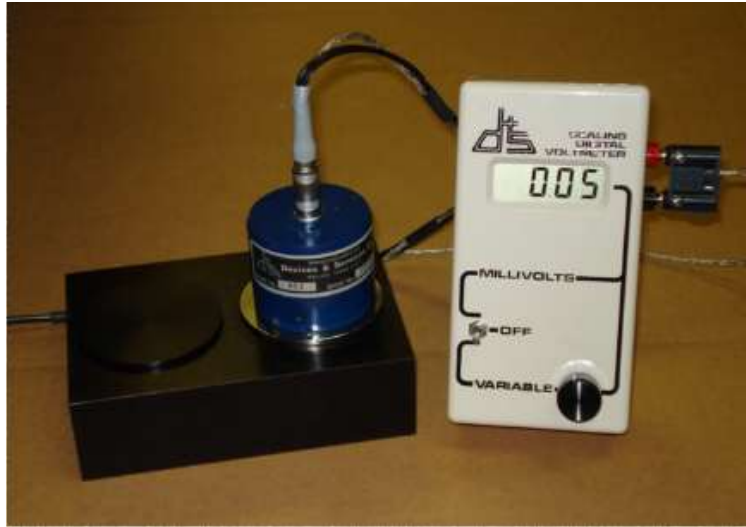
Figure 2.2: Photograph of the emissometer.
