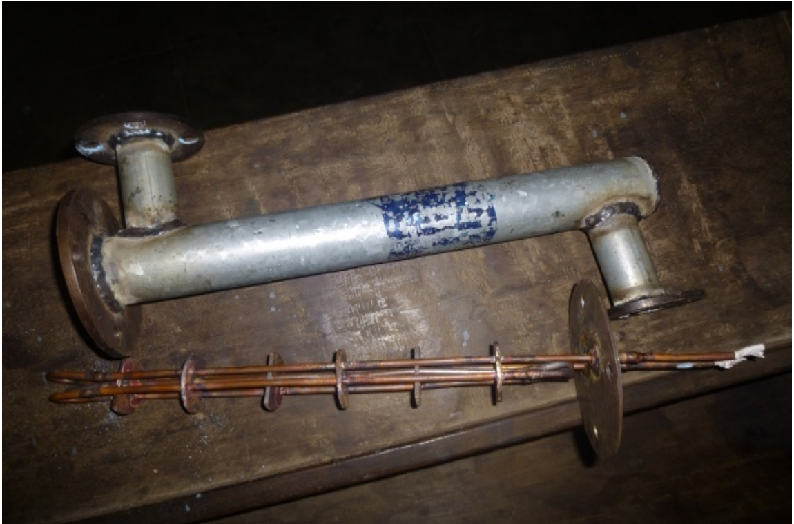
Fig. 4.4 Shell and Tube Heat Exchanger - Inner and Outer Assembly
