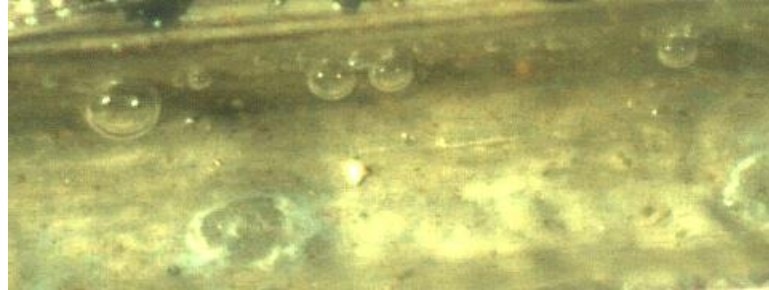
Figure 5.8: Bubble formation of water at Heat flux=90.4 kW/m 2 and mass flux=76.67 kg/m 2 -s.
