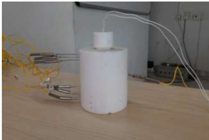
Figure 3.5 Teflon cylinder with thermocouples
