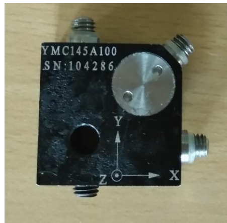
Figure 4.3 Triaxial accelerometer for measuring the vibration
