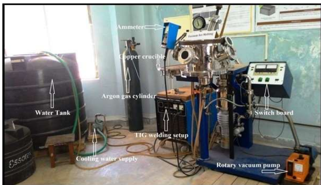
Figure 3.1 Setup of vacuum arc melting furnace
