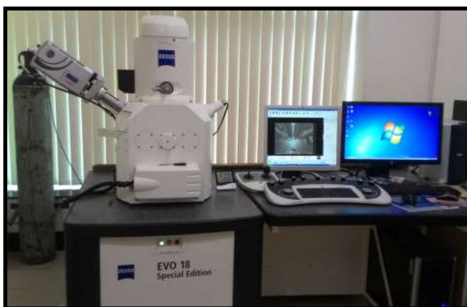
Figure 3.3 Scanning electron microscope with EDAX attachment.
