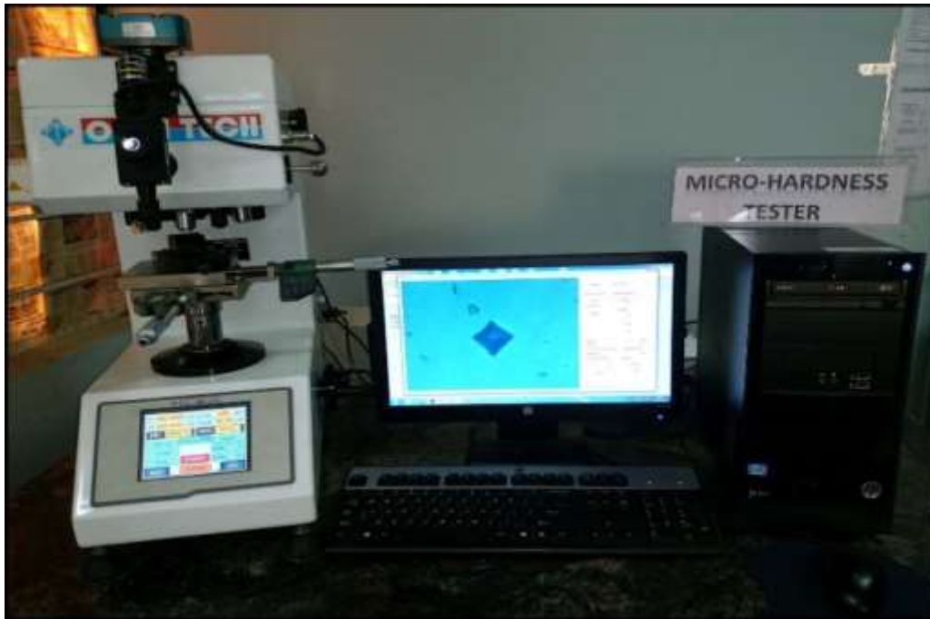
Figure 3.14 Setup of Microhardness testers.
