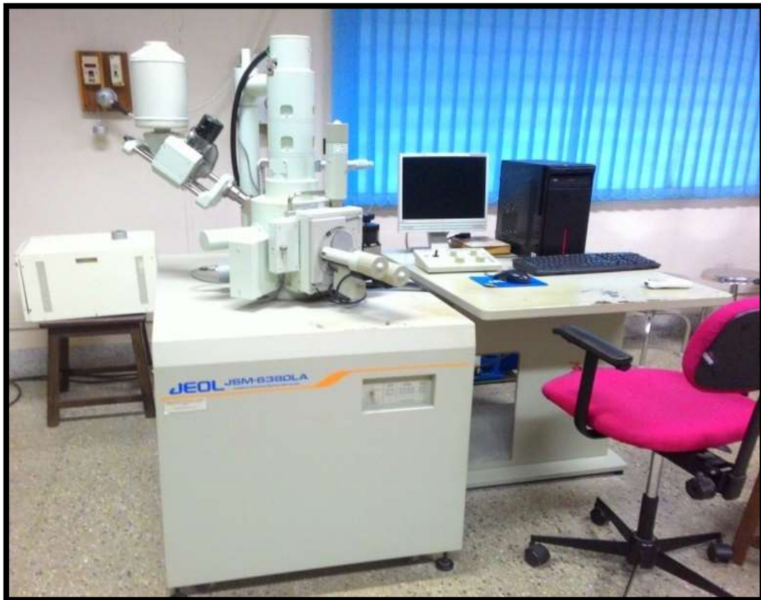
Figure 3.10 Scanning electron microscopy for machines surface morphology.
