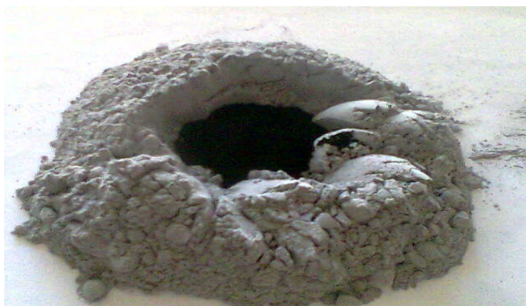
Figure 3.5. Raw powder of Al and CNT before mixing
