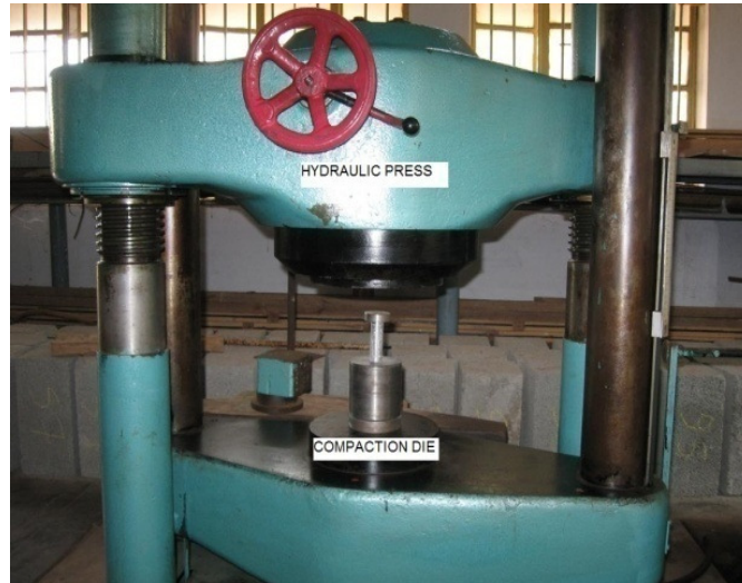
Figure 3.8. Specimen Compaction Setup
