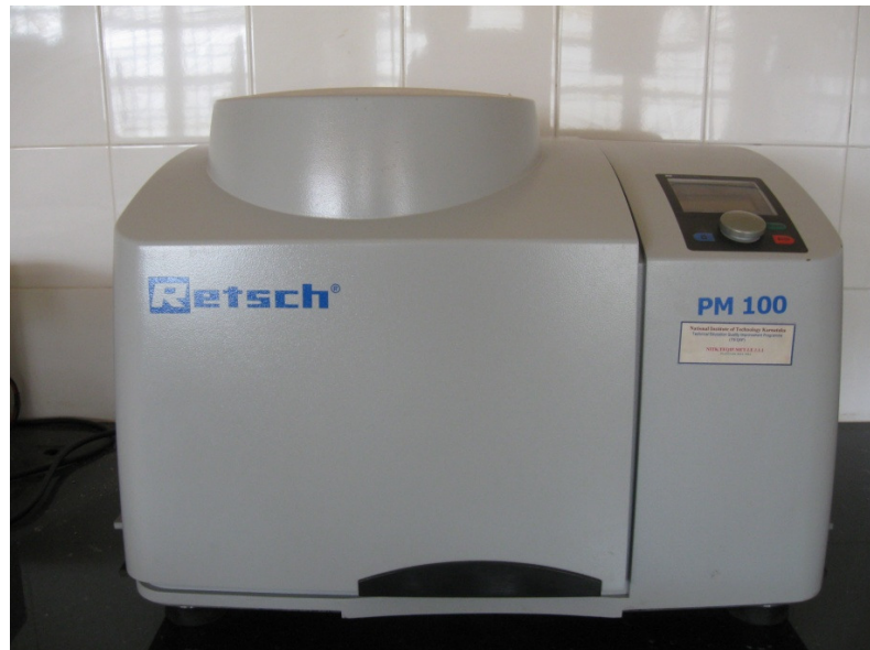
Figure 3.6. High-energy ball milling machine
