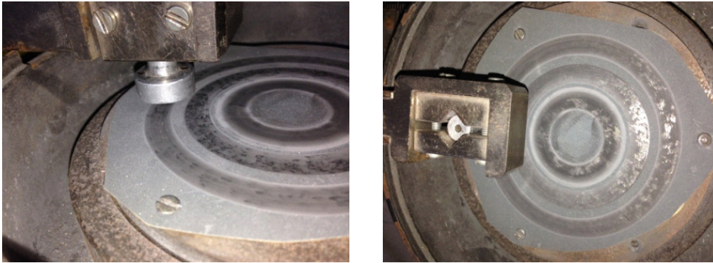
Figure 5.32. Pin on disc set up of wear test machine
