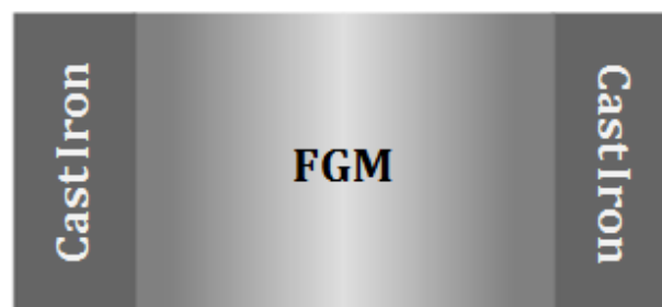
Figure 6.1. Design of brake rotor with FGCL core
