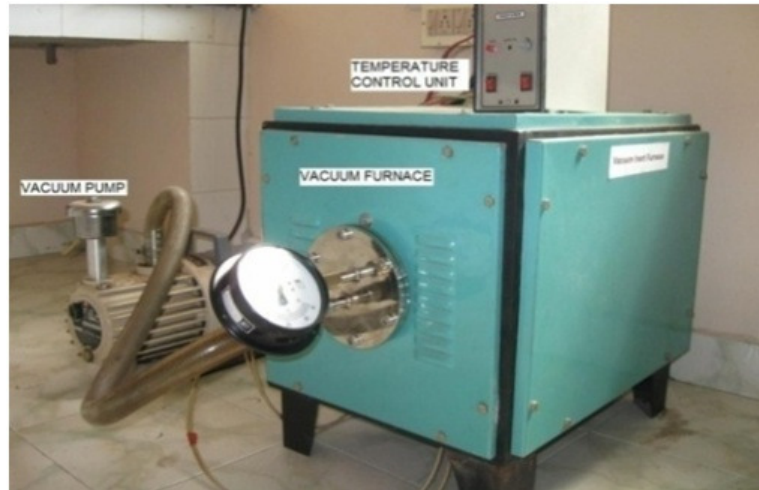
Figure 3.12. Vacuum Furnace used for Sintering
