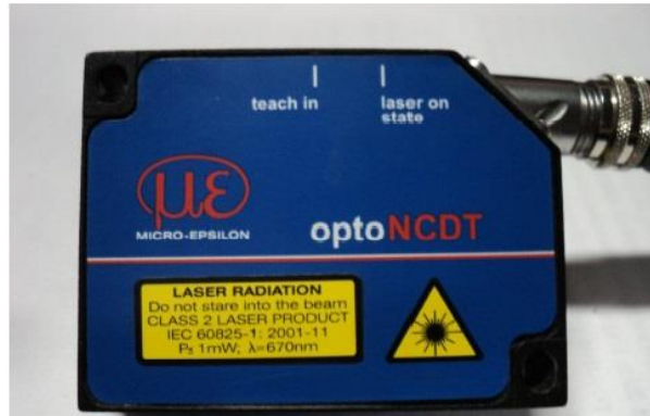
Fig.II.5 Micro epsilon make laser displacement sensor (model: optoNCDT 1402-10).
