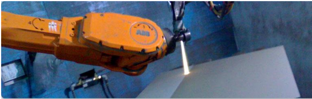
(b) A typical Plasma spraying machine setup ( www.oerlikon.com/metco ).
