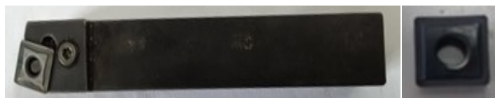
Figure 3. 7 (a) PSBNR 2020 K12 Tool holder (b) AlTiN PVD coated cutting insert.
