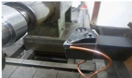
Figure 2. 15 LN 2 supply with SECO tool holder (Bermingham et al., 2011).
