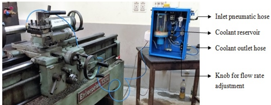
Figure 3. 5 MQL machining experimental setup.
