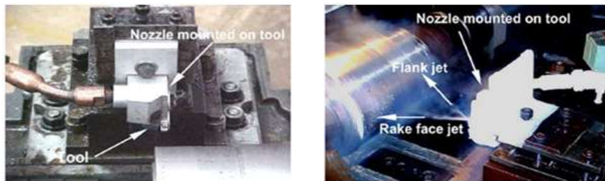
Figure 2. 14 Liquid nitrogen delivery nozzle (Venugopal et al., 2007b).
