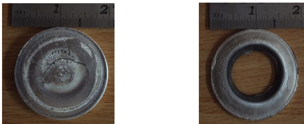
Figure 33. Images showing the of crack developed in aluminum target and a through hole in titanium target due to arcing.
