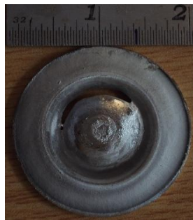
Figure 19. Real sputter crater formed at the time of sputtering of titanium target.
