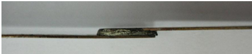
Fig. 5.57: Side view of Cu/solder/Cu lap solder joint
