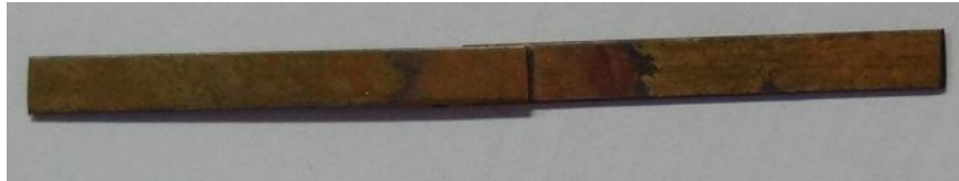
Fig. 5.56: Top view of Cu/solder/Cu and single lap solder joint (top view).
