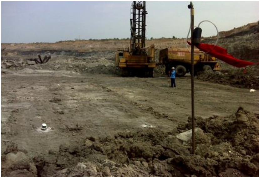
Fig. 3.10 Personal dust monitor near drilling activity in coal benches
