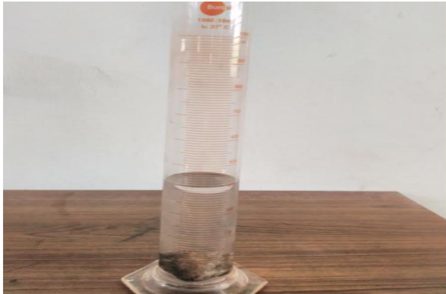
Fig. 3.5 Experimental set up to determine density
