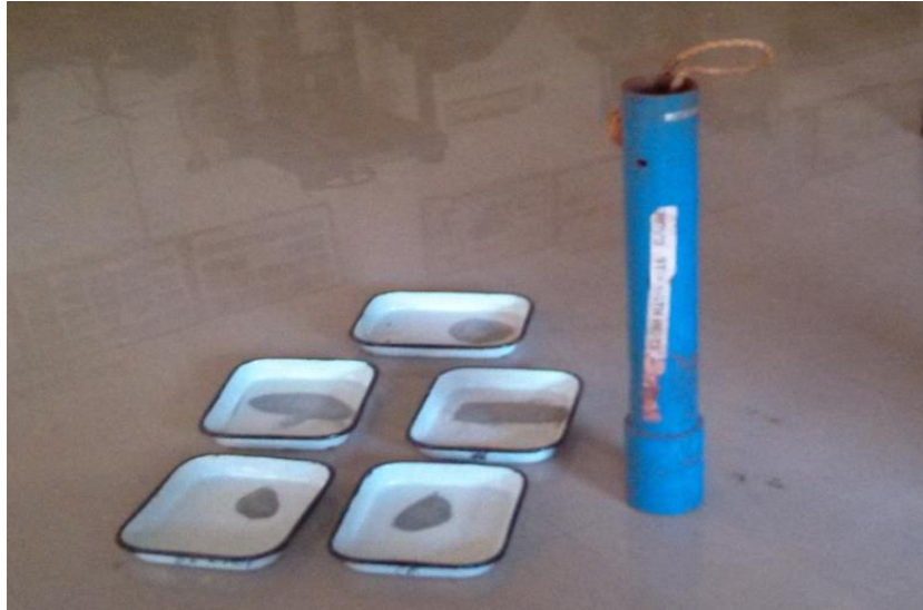
Fig. 3.6 Experimental setup of protodyakonov's strength index
