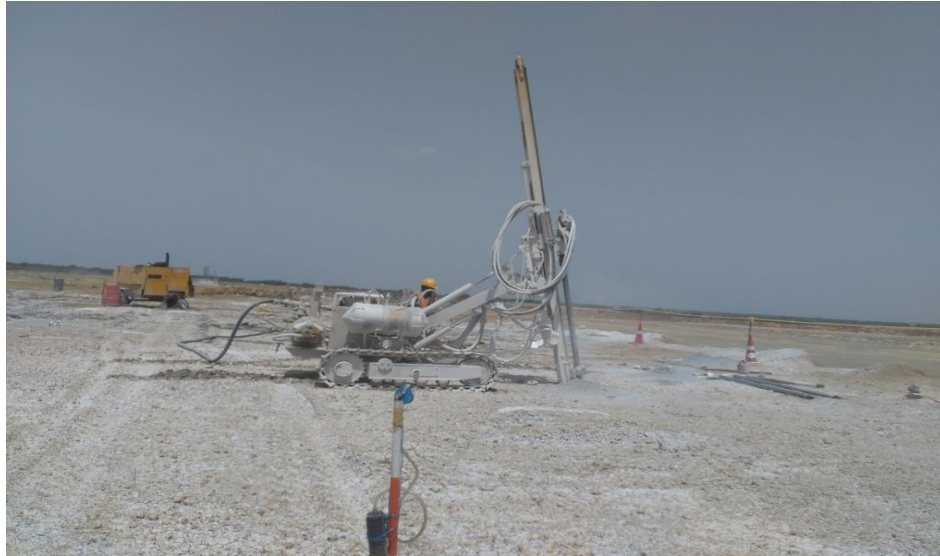
Fig. 3.17 Personal dust monitor near drilling activity in limestone benches
