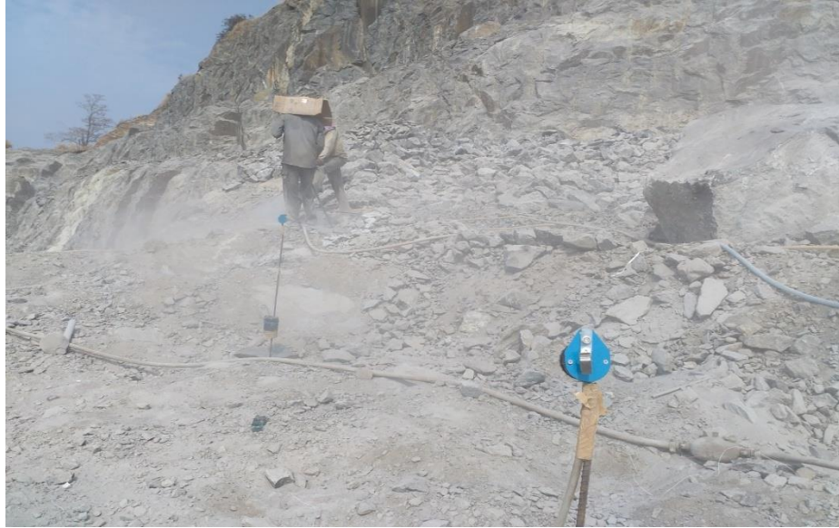
Fig. 3.22 Personal dust monitor near drilling activity in granite quarry
