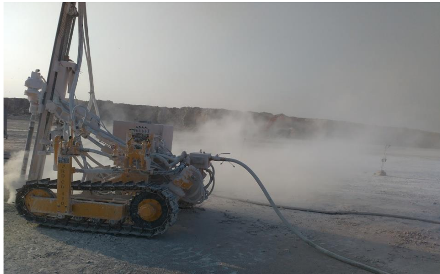
Fig. 3.20 Personal dust monitor near drilling activity in limestone benches
