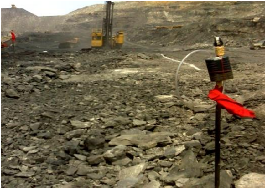
Fig. 3.15 Personal dust samplers near drilling machine in SOP
