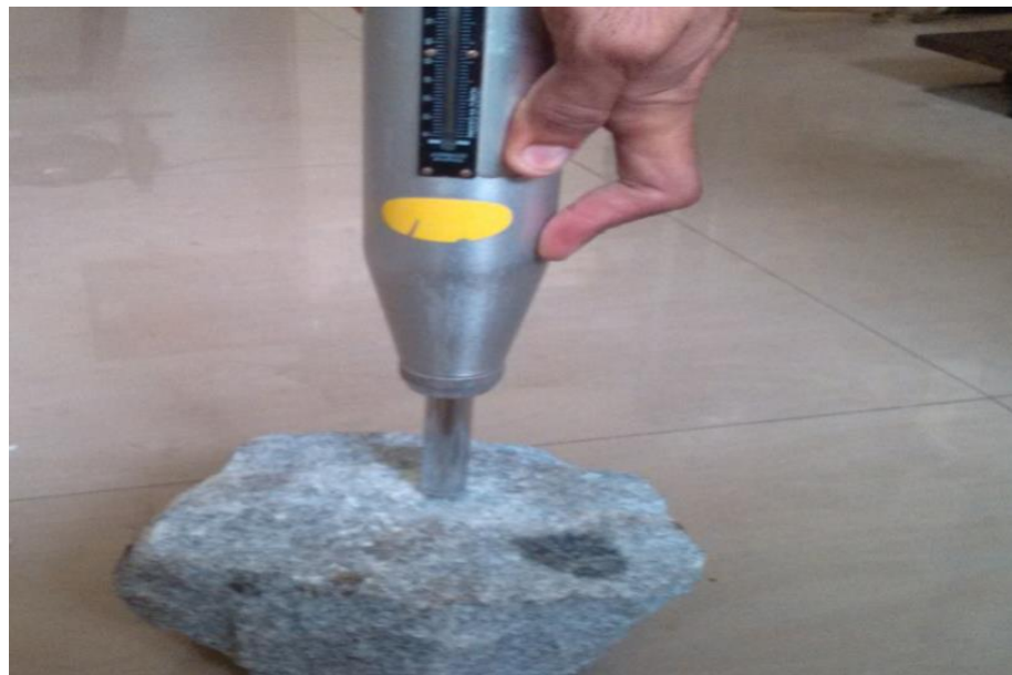
Fig. 3.7 Experimental setup of the Schmidt rebound hardness
