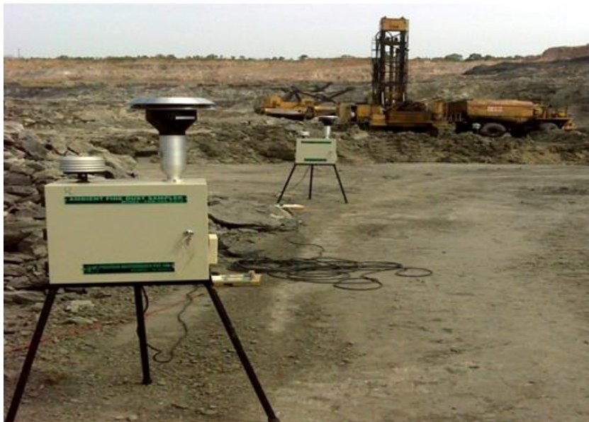
Fig. 3.11 Ambient point samplers near drilling activity in coal benches
