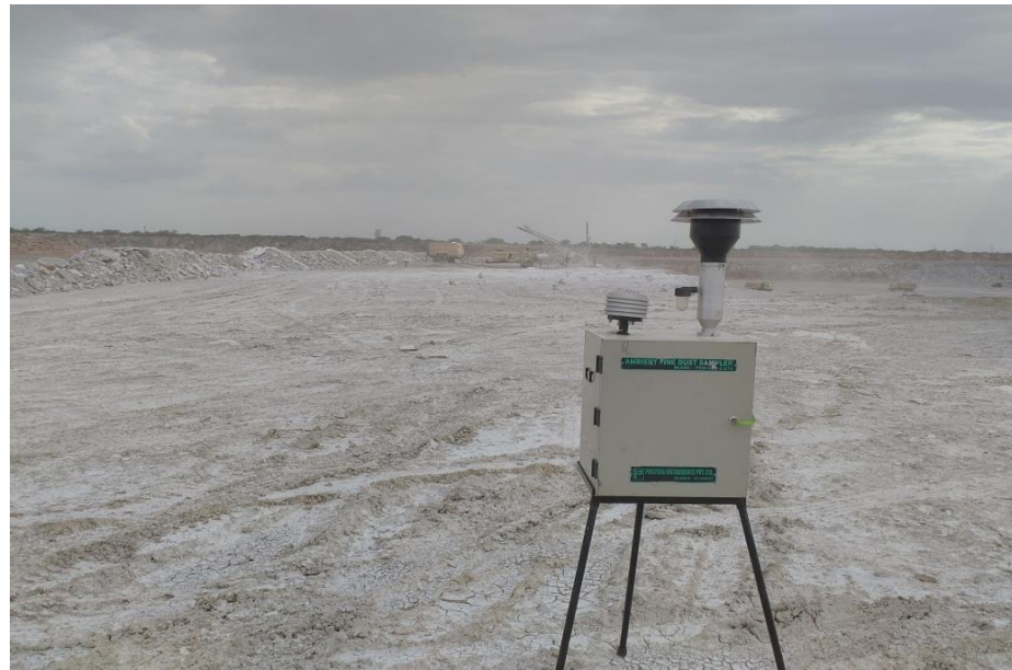
Fig. 3.18 Ambient point dust monitor near drilling activity in limestone benches
