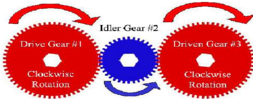
Figure 4.5 Idler gear changes the direction of the driven gear rotation
