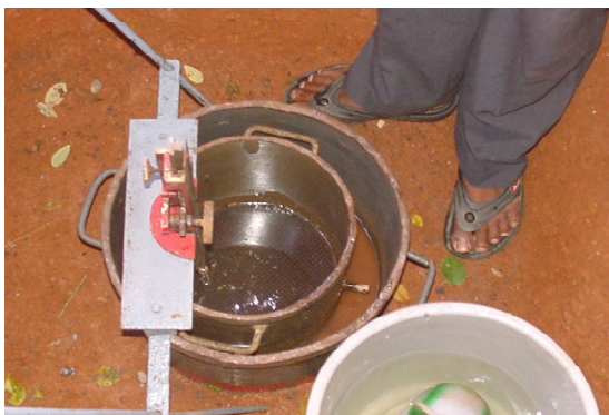
Fig. 3.3 (c) DRI of dia 30 and 15 cm at 1 m Below Ground Level
