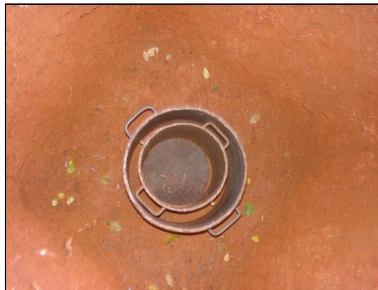
Fig. 3.3 (b) DRI of dia 35 and 25 cm at 1 m Below Ground Level
