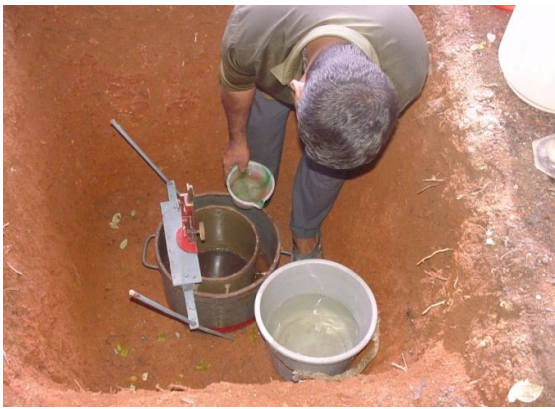
Fig. 3.3 (a) DRI of dia 30 and 15 cm at 1 m Below Ground Level
