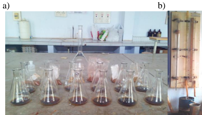
Figure 3.14 Experimental setup of a) Organic matter content test and b) Saturated hydraulic conductivity test
