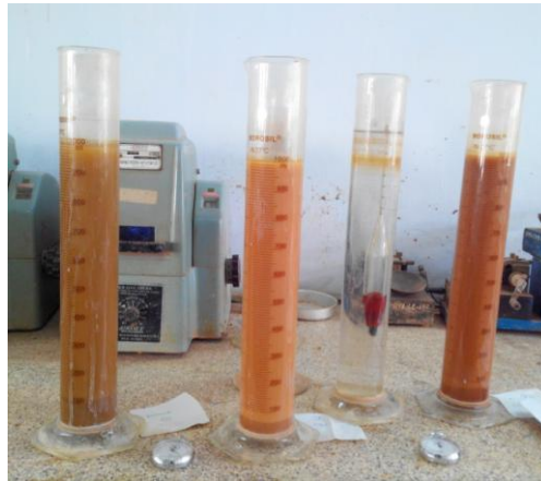
Figure 3.12 Experimental setup of Hydrometer analysis
