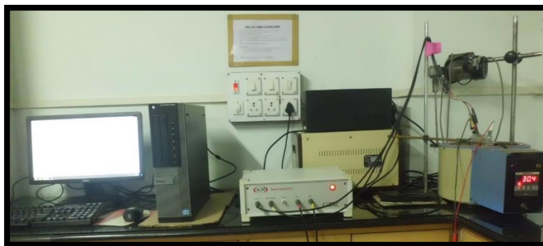
Figure 2.2 The instrumentation setup used for electrochemical measurements.
