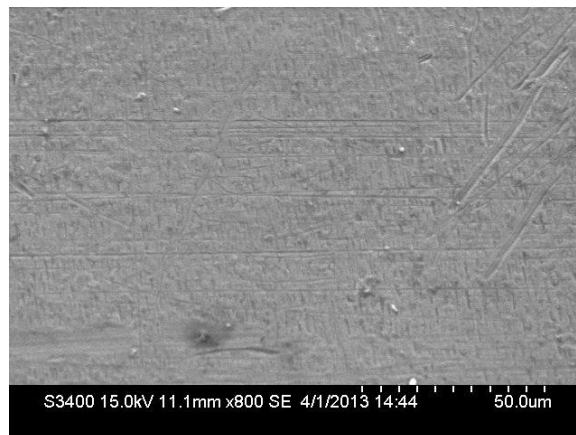
Figure 4.5 SEM image of the surface generated during turning of titanium alloy (Ti-6Al-4V) with PCD insert under MQL condition (cutting speed: 150 m/min, feed: 0.15mm/rev, nose radius: 0.4 mm and depth of cut: 0.5 mm)
