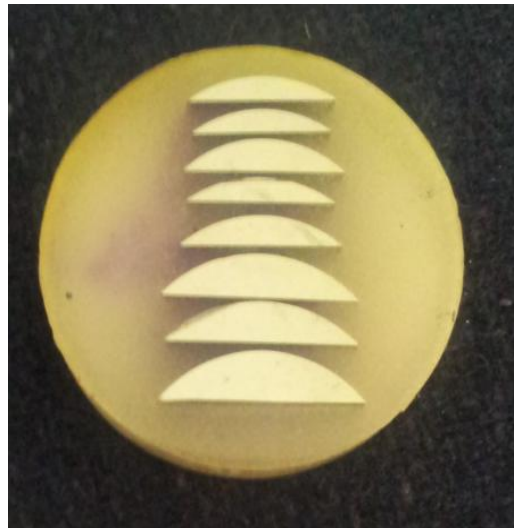
Figure 3.21 Specimen for sub surface hardness and SEM analysis
