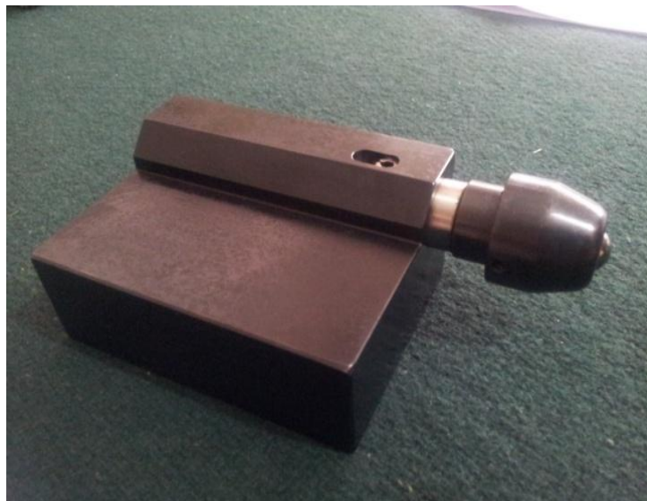
Figure 3.15 Improved ball burnishing tool
