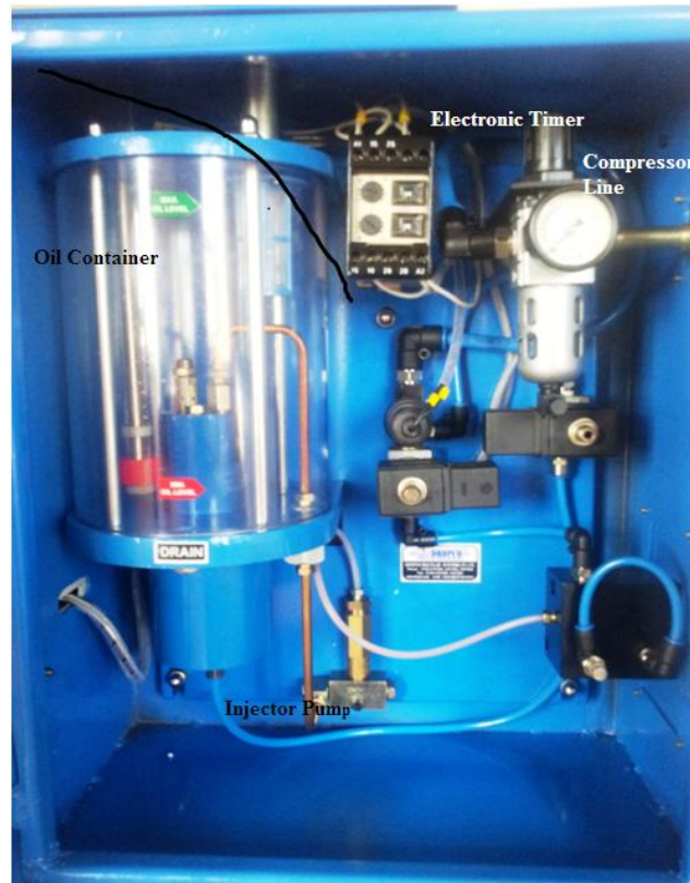
Figure 3.5 Minimum quantity lubrication (MQL) set up
