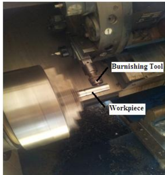
Figure 3.13 Experimental set up of burnishing experiments
