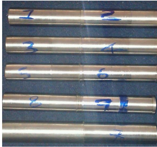
Figure 3.18 Titanium bars used in the ball burnishing experiments for wear tests
