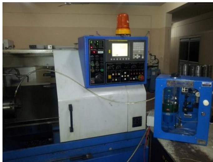
Figure 3.10 CNC lathe and MQL setup used for turning and burnishing experiments
