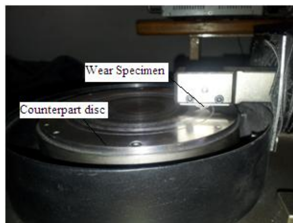
Figure 3.20 Experimental set up for wear tests with specimen
