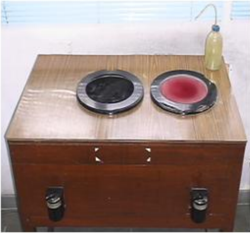
(b) Rotary Abrasive Polishing Equipment (c) Diamond Paste With Polishing Cloth Equipments for Surface Preparation
