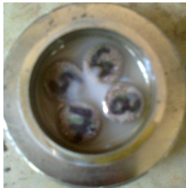
Test Specimens Mounted using Denture Based Polymer
