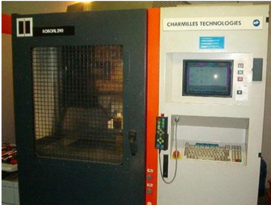
WEDM (ROBOFIL 290) used for Machinability Studies
