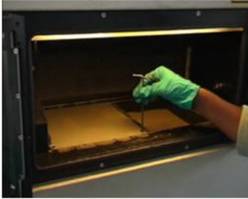
Mounting and Leveling of Base Plate in EOSINT M250 DMLS Machine
