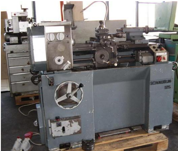
(a) Tool Room Lathe
