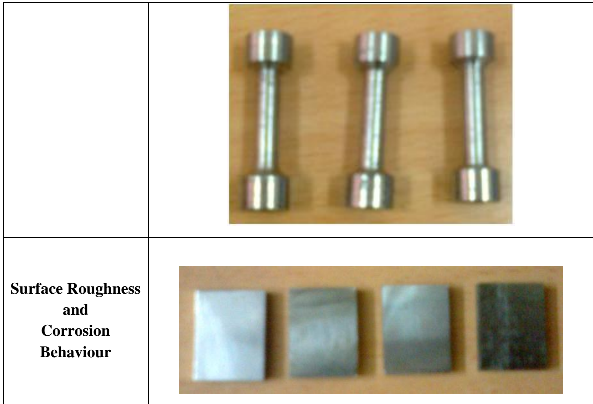
Figure 5.19 Test Specimens Produced by DMLS Process
