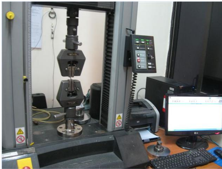
INSTRON-5569 Loaded with Test Specimen
