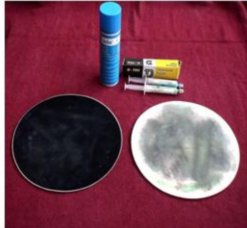
(b) Rotary Abrasive Polishing Equipment (c) Diamond Paste With Polishing Cloth Equipments for Surface Preparation
