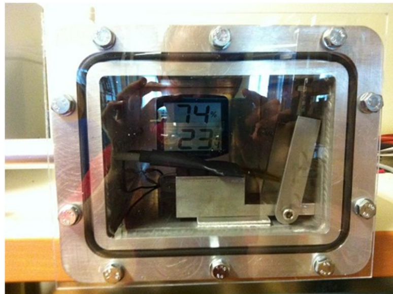
Figure 4.2.6 Experimental set up for thermal property measurement at various relative humidity levels
