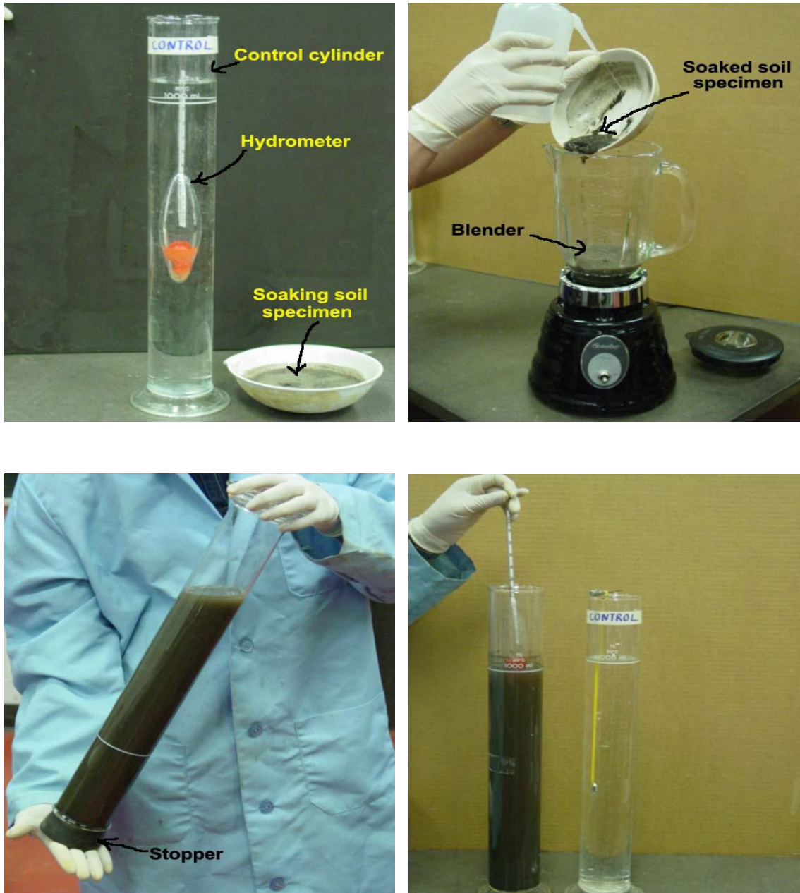
Figure 3.5: Experimental set up for hydrometer analysis
