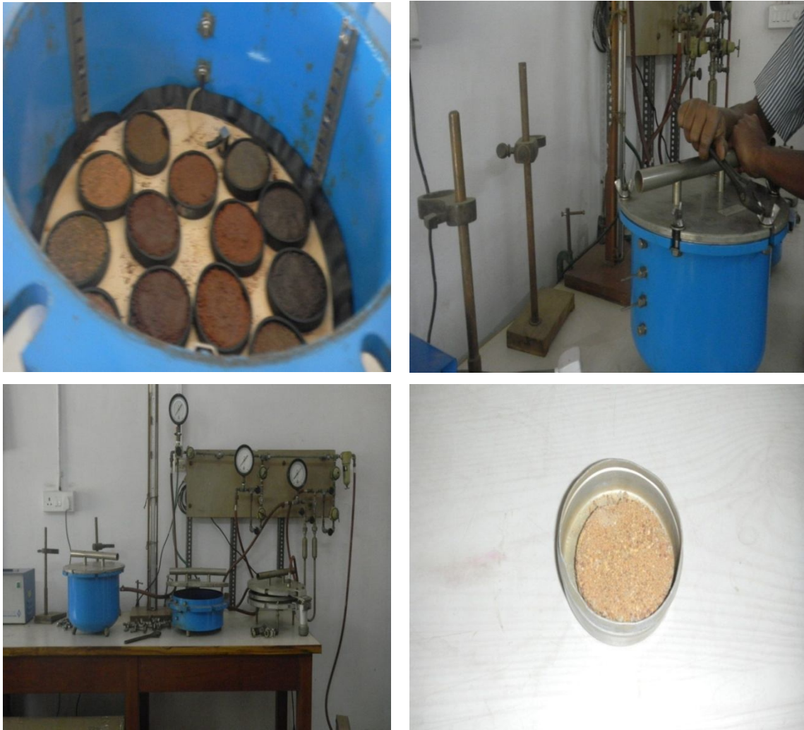
Figure 3.9: Experimental set up of Pressure plate apparatus
