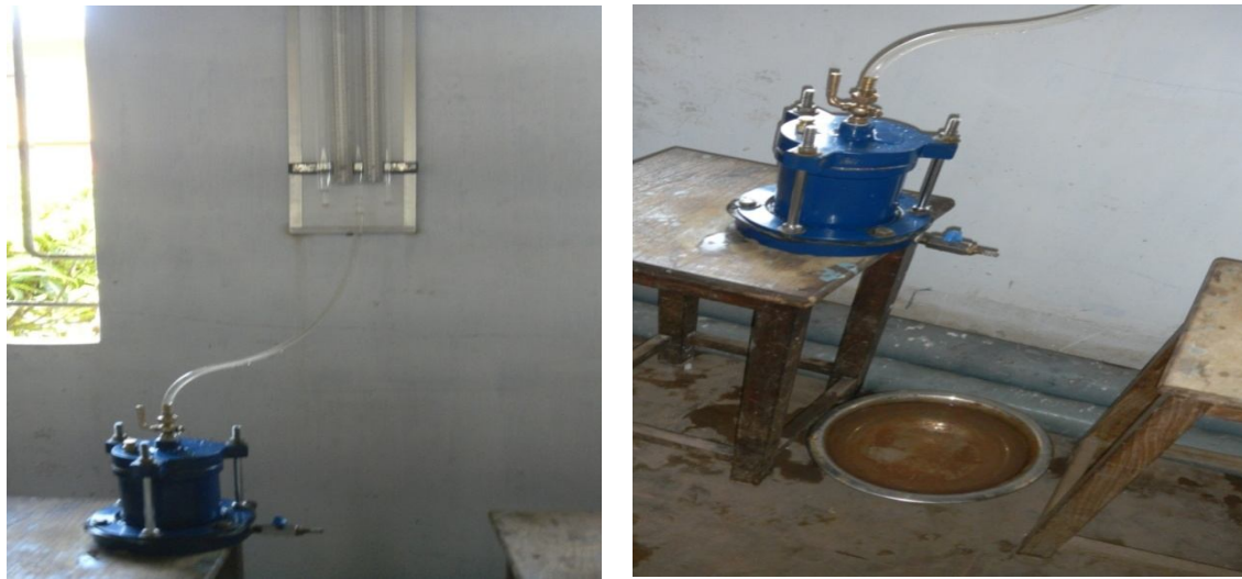
Figure 3.8: Experimental set up for falling head test
