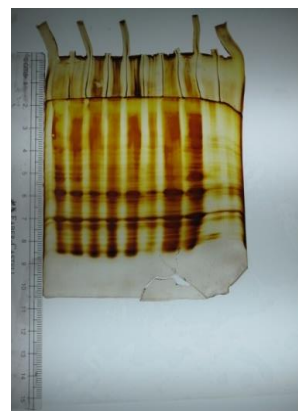
Fig. 4.29 Silver staining SDS PAGE (10-17%) of cell wall proteins by Pitarch et al. (2002) method
