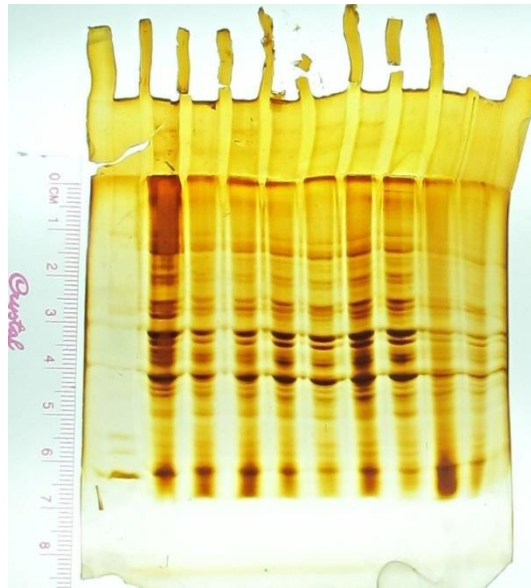
Fig. 4.33. SDS PAGE (12-17%) of samples from first lane standard protein molecular weight marker followed by cell wall protein samples from RL-13, RL-29, CL-01,RL-06, CN-67, RL-03, CN-181, RL-09, CN-192 (Silver stained)
