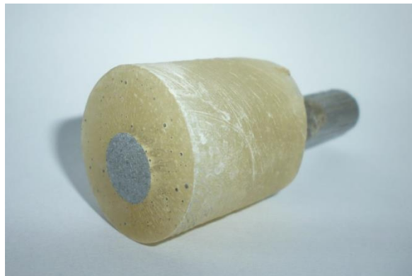
Fig. 2.1 Alloy specimen mounted in epoxy resin.
