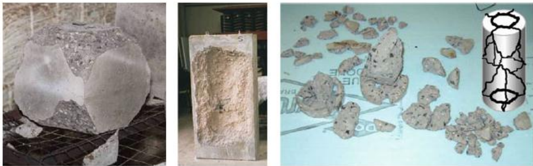
(a) Corner spalling (b) Surface spalling (c) Explosive spalling
