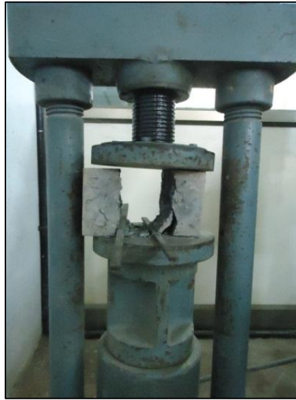
Fig 3.10: Splitting tensile strength test
