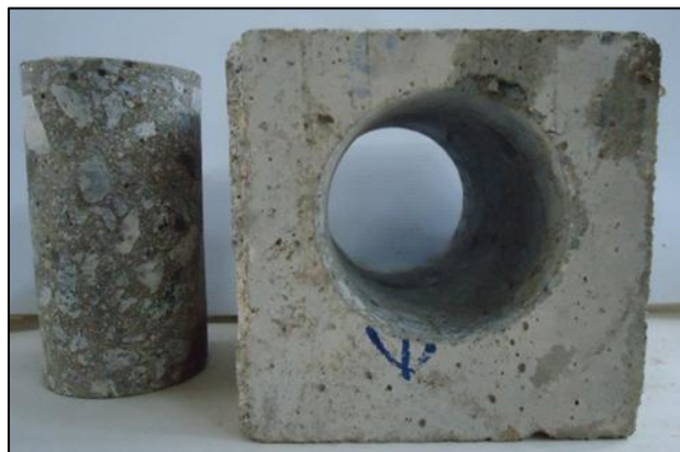
Fig. 3.16: Concrete core extracted from cube specimen
