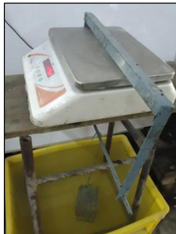
Fig. 3.7: Submerged weight measurement set up
