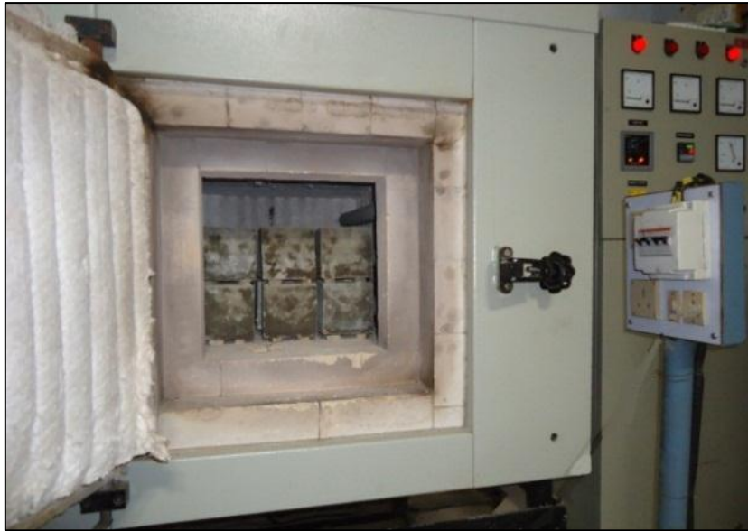
Fig. 3.4: Muffle furnace and arrangement of specimen for exposure
