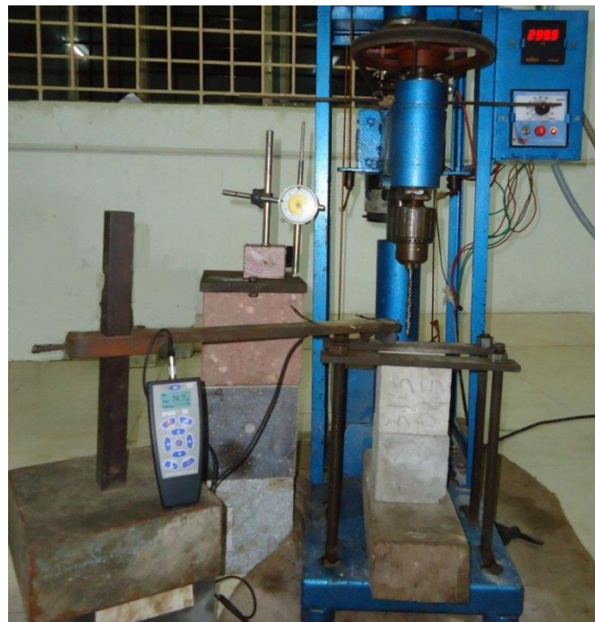
Fig 3.13: Test setup for determination of drilling time (Source: Mining Engineering Department, NITK, Surathkal)
