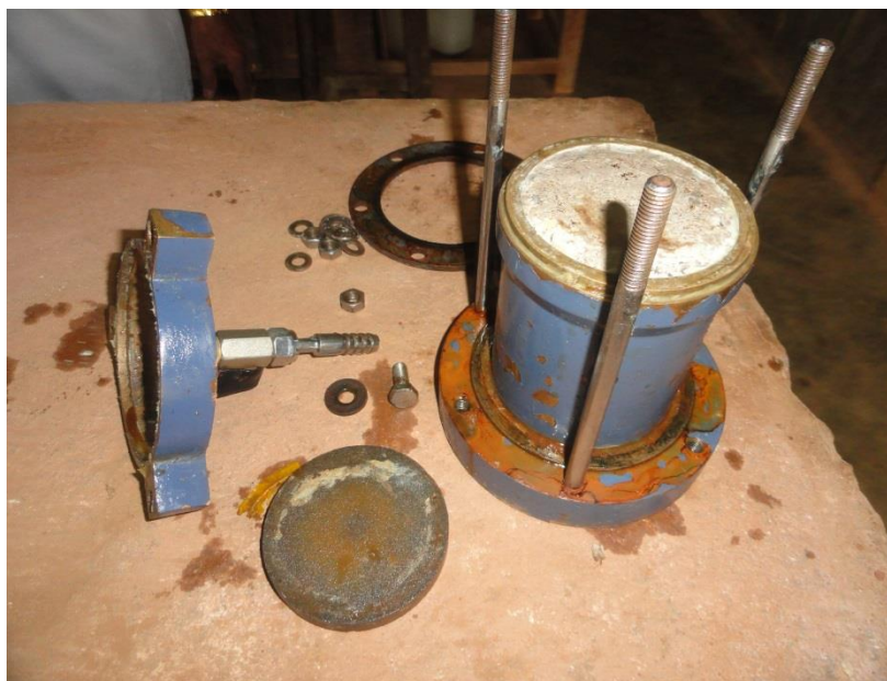
Fig 4.3 Apparatus used for the permeability tests
