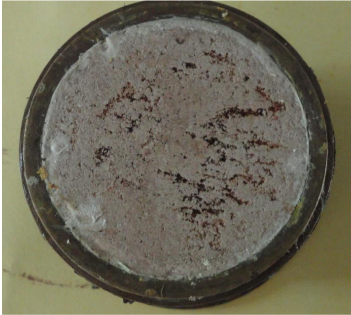
Fig 7.1 Formation of precipitates from pollutants in the soil due to leachate flow
