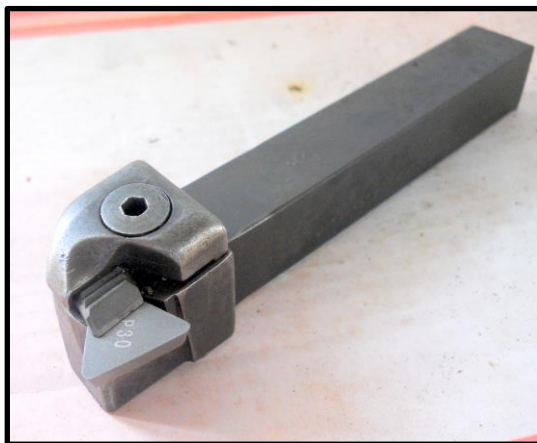
Figure 3.3: Carbide insert with a general purpose ISO tool holder CTLPR2020L16
