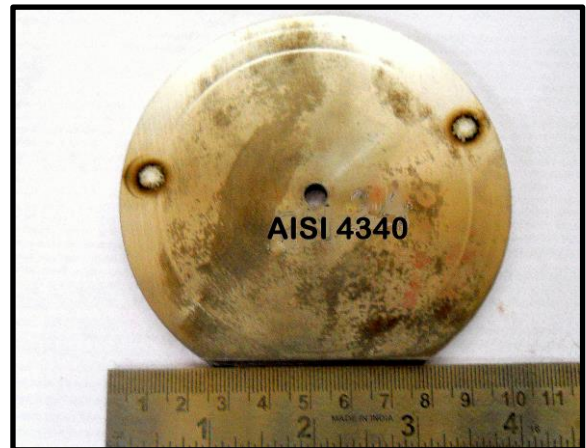
Figure 3.4: Work piece showing the spectrometric analysis location.
