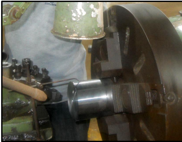
Figure 3.2: Work piece preparation and set up prior to machining on a four jaw chuck of a HMT-Lathe.
