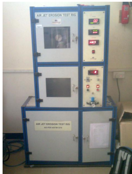
Fig. 3.2 Schematic view of an air jet erosion test rig.
