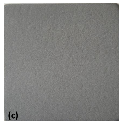
Fig. 4.5 Optical macrograph of 25%(Cr 3 C 2 -25(Ni 20 Cr)) + 75%NiCrAlY coated materials. Sample size is 25 mm X 25 mm (a) Ti-31 (b) Superco-605 (c) MDN-121
