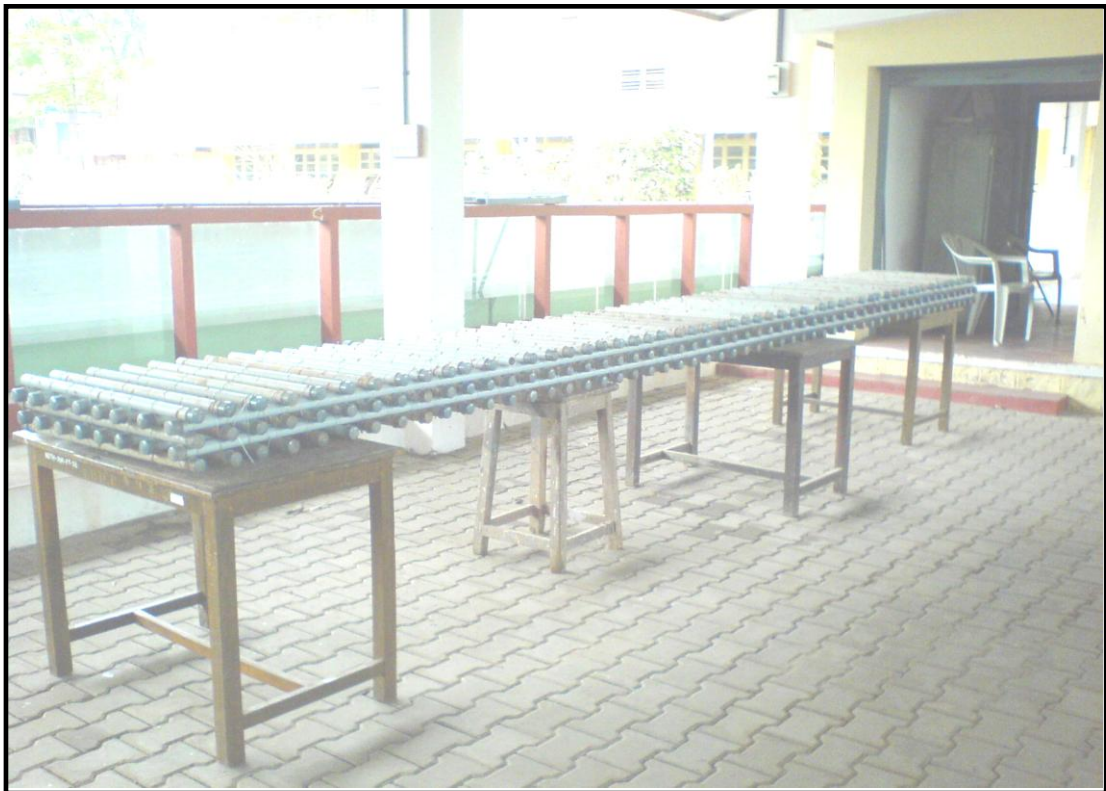
Plate 3.2 View of the floating pipe breakwater model with five layers of pipes and S/D = 5 (Jagadisha, 2007)
