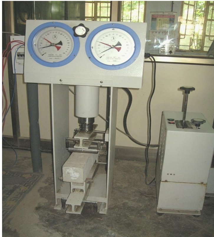
Fig 3.6 Flexural Test by Third Point Loading
