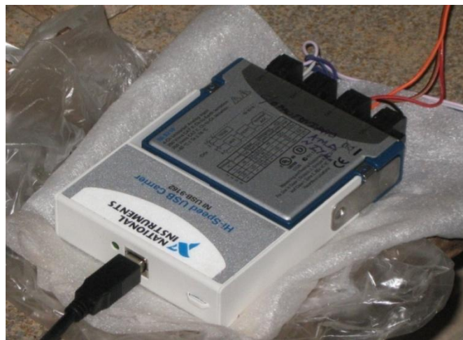
Fig 6.5 Data Acquisition Unit
