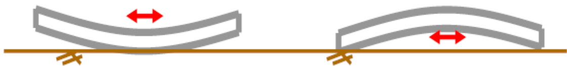
Fig 2.3 Upward and downward curling of concrete pavement
