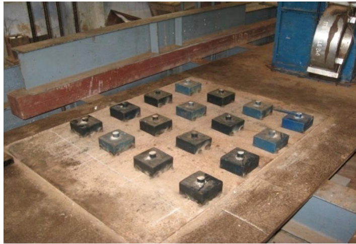
Fig 6.4 Arrangement of box springs
