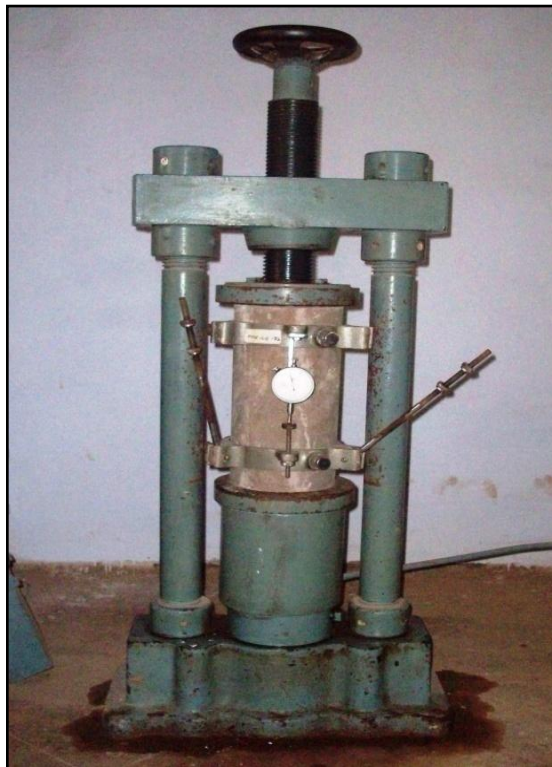
Fig 3.7 Determination of Modulus of Elasticity
