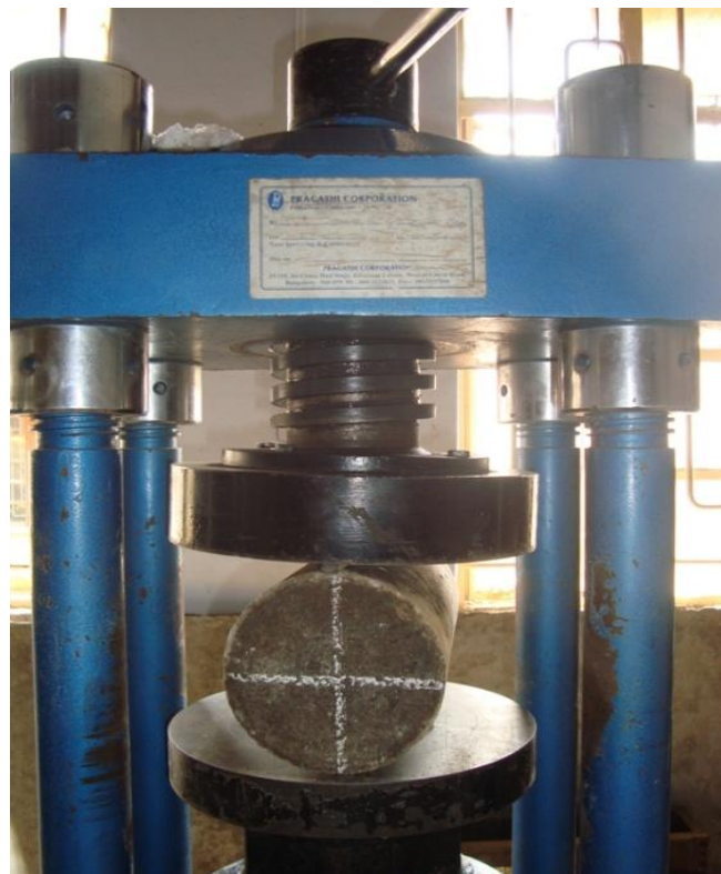
Fig 3.5 Splitting Tension Test
