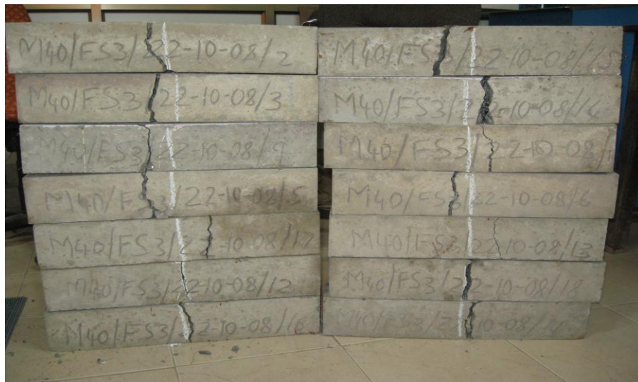
Fig 4.7 Failed specimens (FS3)
