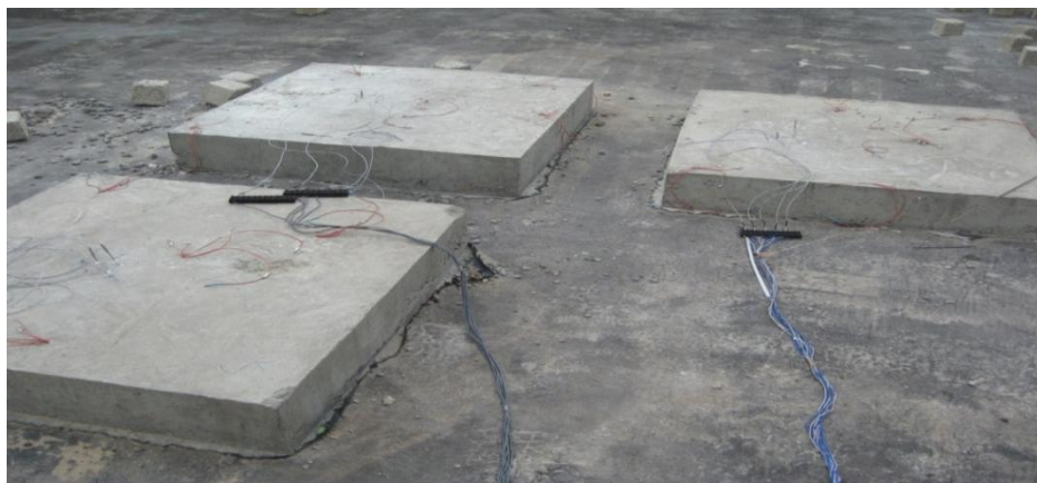
Fig 5.5 Test slabs with temperature sensors
