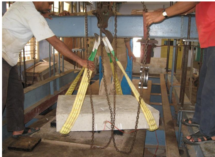
Fig 6.7 Placing of slab over steel box springs
