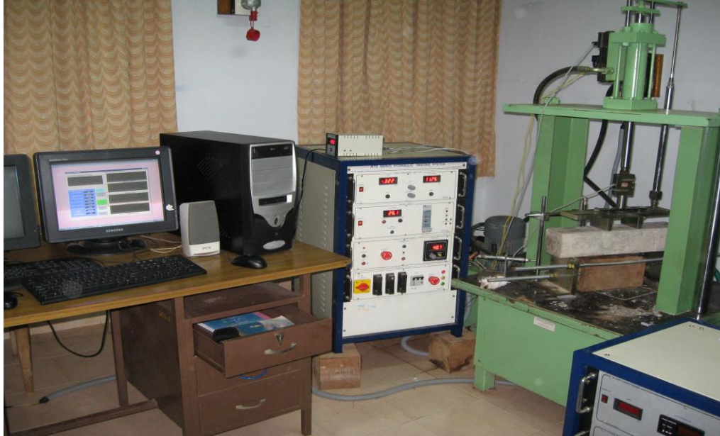
Fig 4.3 Accelerated Fatigue (repeated load) test set up
