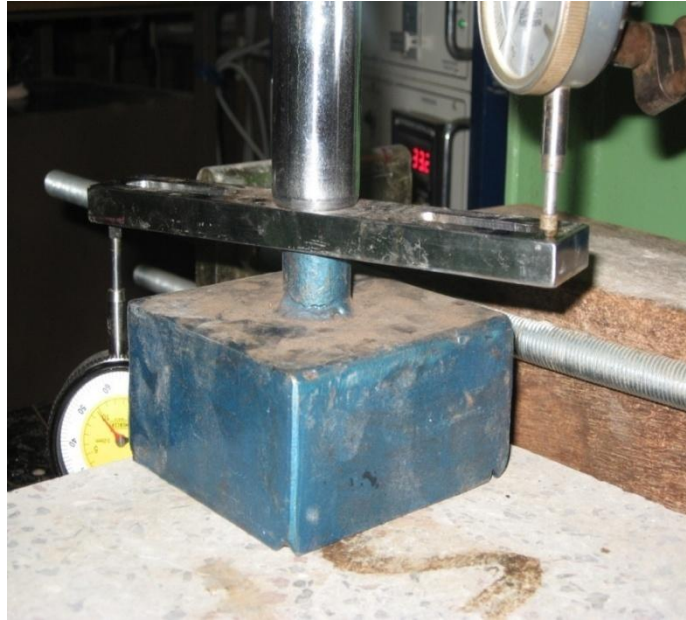
Fig 6.1 Testing arrangement for stiffness of steel box
