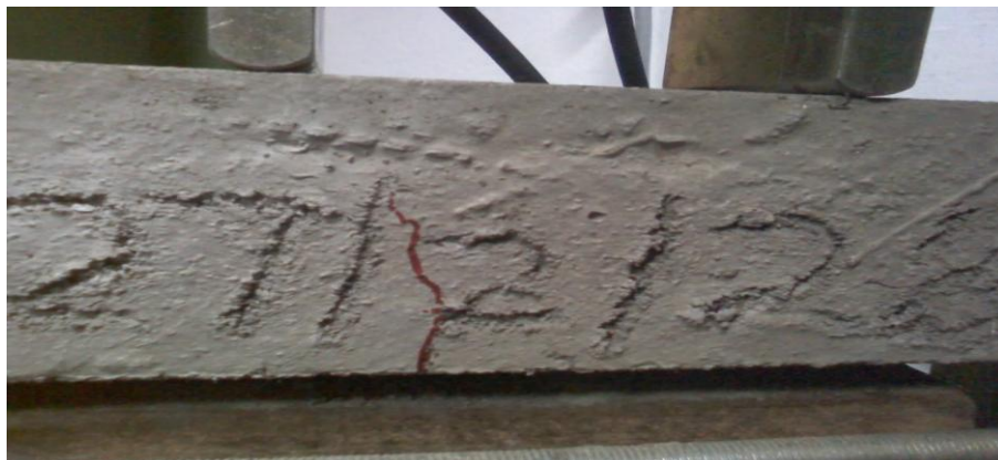
Fig 4.5 Crack propagation during flexural fatigue test
