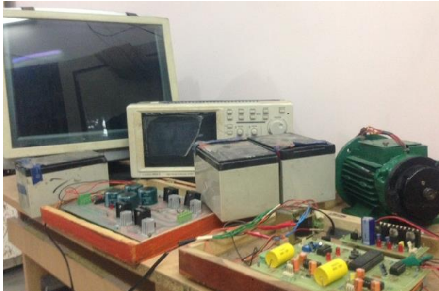
Fig.4.5 Test bench for flux linkage curves
