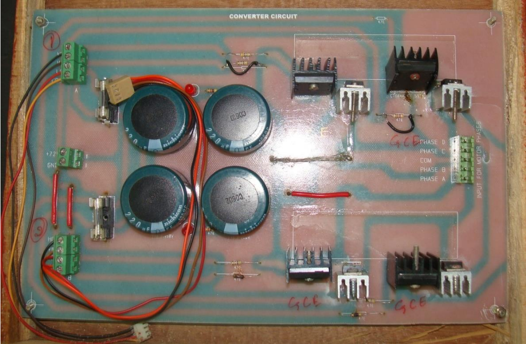
(f) Converter Circuit
