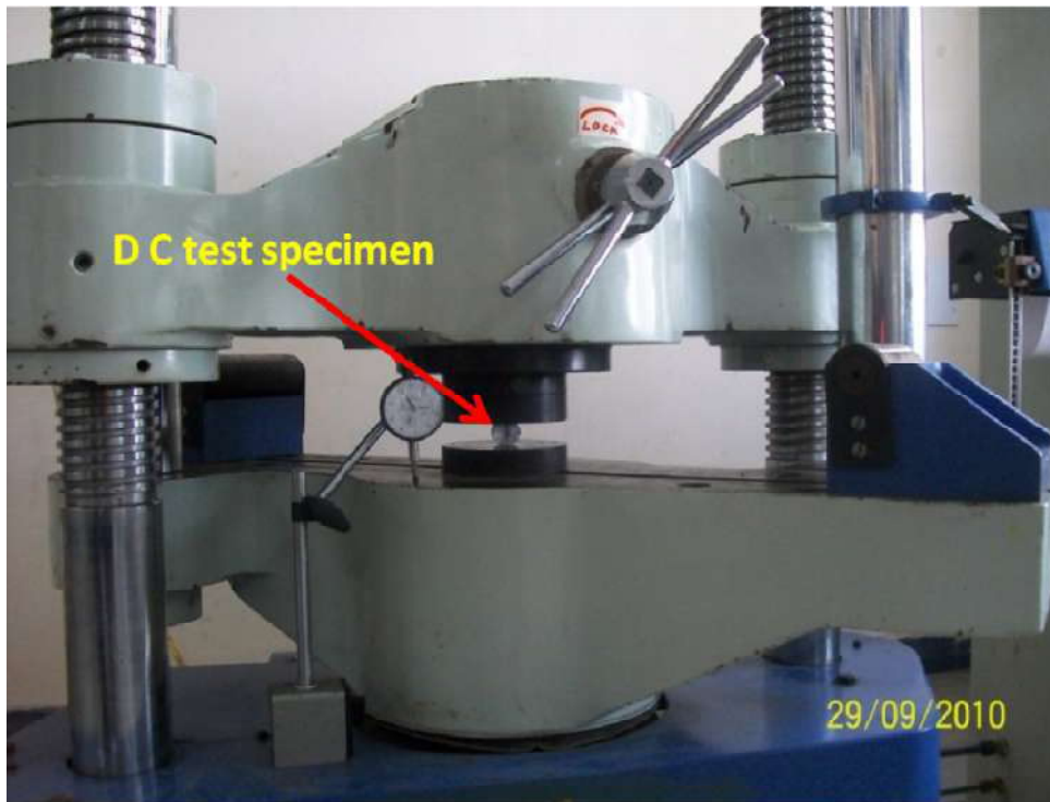
Fig. 3.13 UTM with application of Diametral compressive load
