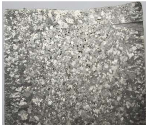
Fig. 4.26 The macrostructure of the as-cast specimen
