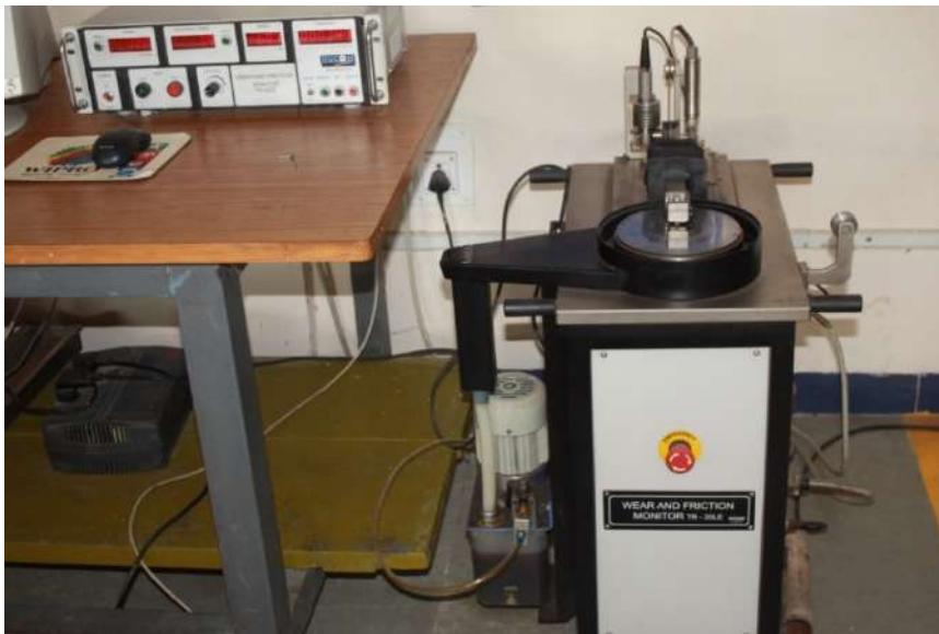
Fig. 3.10 Pin-on-Disc Wear testing Machine
