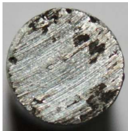
Fig. 4.103 Pin surface with oxide film
