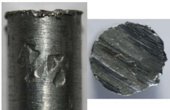
Fig. 4.100 Large sheets in the wear debris from the spalling of transferred pin material on the wear track
