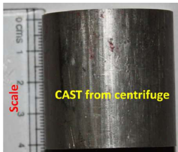
Fig. 3.5 Centrifugally Cast Specimen
