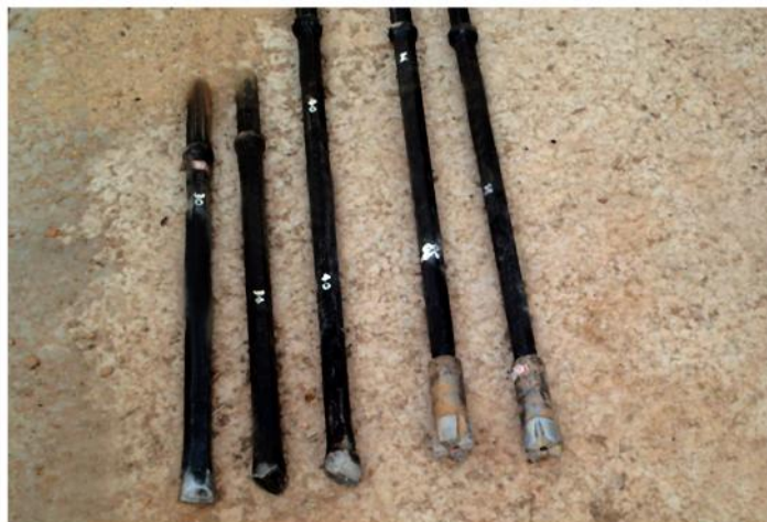
Fig. 4.7 Drill Bits used in laboratory drilling experiments (Integral and threaded)
