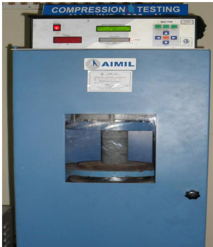
Fig. 4.2 AIM-317E-Mu Compression testing machine (AIMIL, New Delhi)
