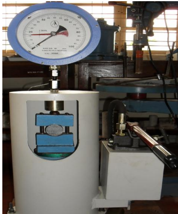
Fig. 4.4 Tensile strength testing machine (AIMIL, New Delhi)
