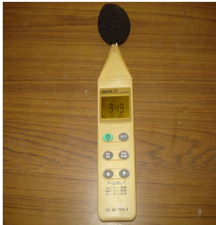
Fig.4.6. Model 320, IEC 651 Type II sound level meter
