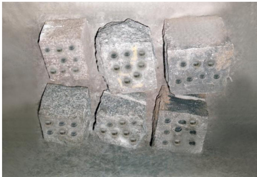
Fig. 4.8 View of some of the Rock Blocks used in laboratory drilling experiments (Integral chisel and threaded cross bit)
