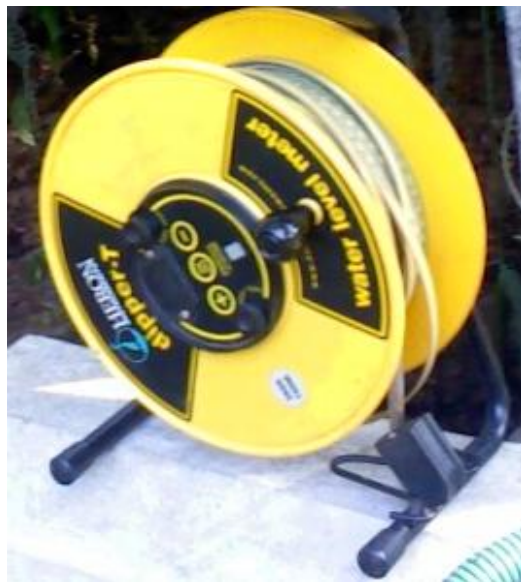
Figure 3.7 Groundwater level measuring instrument-Dipper-T
